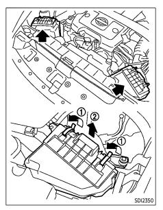
Remove the retainers  $\ensuremath{\mathbb{T}}$  as illustrated and pull out the filter element  $\ensuremath{\mathbb{T}}$  .
