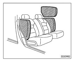
FRONT SEAT-MOUNTED SIDE-IM-PACT AND ROOF/DOOR-MOUNTED CURTAIN SIDE-IMPACT AND ROLL-OVER (if so equipped) SUPPLEMEN-TAL AIR BAG SYSTEMS
