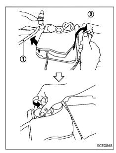
2. Take the hose ① and the power plug ② out of the air compressor. Remove the cap of the bottle holder from the air compressor.
