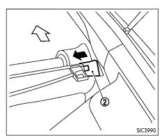
To remove the cargo cover unit, stow the cover and pull the holder ② to the opposite side.
