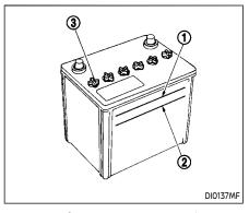
Check the fluid level in each cell (Remove the battery cover if it is necessary). It should be between the UPPER LEVEL ① and LOWER LEVEL ② lines.
