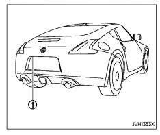
To display the rear view, the RearView Monitor system uses a camera located iust above the vehicle's license plate (1).
