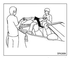
c. Pull up the storage lid from the left and right side of the vehicle by hand.
