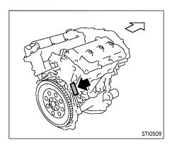
**ENGINE SERIAL NUMBER** The number is stamped on the engine as shown.
