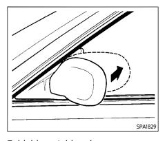
Foldable outside mirrors Fold the outside mirror by pushing it toward the rear of the vehicle.
