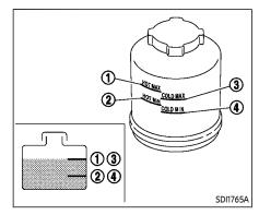
Check the fluid level in the reservoir.
