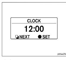
3. Push the **u** switch (a) for a short time to complete the clock adjustment.
