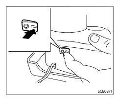
6. Push the ignition switch to the "ACC" position. Then turn the compressor switch to the ON (-) position and inflate the tire up to the pressure that is specified on the tire and loading information label affixed to the driver's side center pillar if possible, or to the minimum of 26 psi (180 kPa). Turn the air compressor off briefly in order to check the tire pressure with the pressure gauge.
