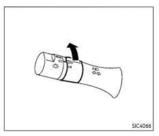
FOG LIGHT SWITCH (if so equipped) To turn on the rear fog light, turn the
