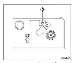
Mark the center of the hole ® on both sides with a felt-tip pen. Remove the bracket from the bumper, and then open 0.9 to 1.0 inch (22 to 25 mm) diameter holes on the bumper using the marks ® as a center.
