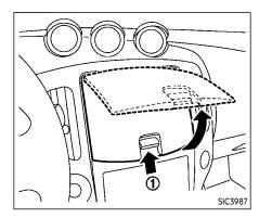
INSTRUMENT POCKET (except for navigation system equipped models)
