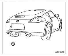
If dirt, rain or snow accumulates on the camera ①, RearView Monitor may not display objects clearly. Clean the camera by wiping it with a cloth dampened with a diluted mild cleaning agent and then wiping it with a dry cloth.
