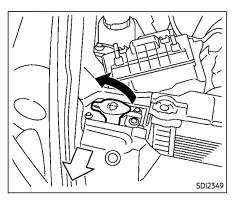
Fill the window washer fluid reservoir periodically. Add window washer fluid when the low window washer fluid warning appears.
