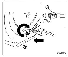
Remove the protective cap (A) of the hose and screw the hose securely onto the tire valve. Make sure that the pressure release valve (B) is securely tightened. Make sure that the air compressor switch is in the OFF (○) position, and then insert its power plug into the power outlet in the vehicle.
