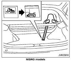
Top tether anchor point location The anchor point is located on the floor of the cargo area.
