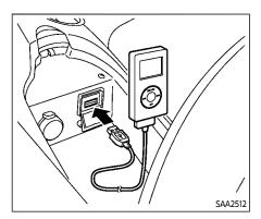
Open the console lid and connect the iPod® cable to the USB connection port. If compatible, the battery of the iPod® is charged while the connection to the vehicle.
