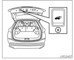
Power operation is available when in the OFF position by the instrument panel switch and the key fob button.
