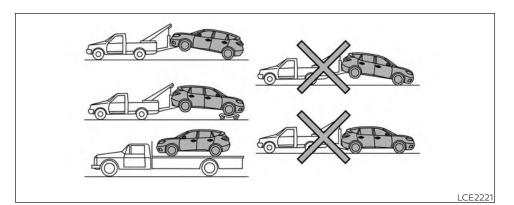
Front-Wheel Drive (FWD) models with Continuously Variable Transmission (CVT)
