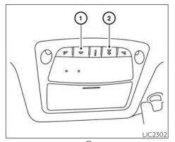
When the ON switch (1) is pushed, the footwell lights (if so equipped), step lights (if so equipped), map lights and rear personal lights will automatically turn on and stay on for a period of time when:
