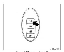
Type A (if so equipped) The  $\Omega$  button will be on the NISSAN Intelligent Key® if the vehicle has Remote Engine Start. This feature allows the engine to start from outside the vehicle
