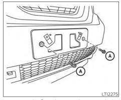
To mount the front license plate, attach the license plate bracket to the plastic finisher at the location marks (small dimples) using the two provided screws (A).
