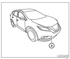
The I-FCW system uses a radar sensor (A) located behind the lower grille of the front bumper to measure the distance to the vehicle ahead in the same lane.
