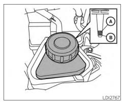
Check the fluid level in the reservoir
