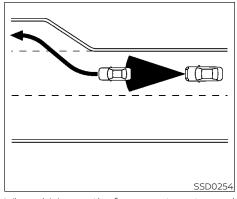
When driving on the freeway at a set speed and approaching a slower traveling vehicle ahead, the ICC system will adjust the speed to maintain the distance, selected by the driver, from the vehicle ahead. If the vehicle ahead changes lanes or exits the freeway, the ICC system will accelerate and maintain the speed up to the set speed. Pay attention to the driving operation to maintain control of the vehicle as it accelerates to the set speed.
