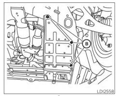
4. Remove pins **(B)** from the underengine protector.
