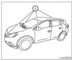
the cameras (1), the MOD system may not operate properly. Clean the camera by wiping with a cloth dampened with a diluted mild cleaning agent and then wiping with a dry cloth.
