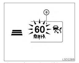
When passing another vehicle, the set speed indicator (B) will flash when the vehicle speed exceeds the set speed. The vehicle detect indicator will turn off when the area ahead of the vehicle is open. When the pedal is released, the vehicle will return to the previously set speed.
