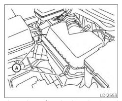
The air cleaner filter should not be cleaned and reused. Replace it according to the maintenance log shown in the "Maintenance and schedules" section of this manual
