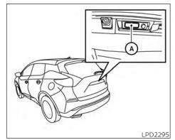
When the power liftgate main switch is pushed to the OFF position, the power operation is not available by the liftgate opener switch (A) or liftgate close switch (B) on the liftgate.
