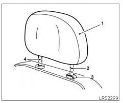
NON-ADJUSTABLE HEAD RESTRAINT/HEADREST **COMPONENTS**
