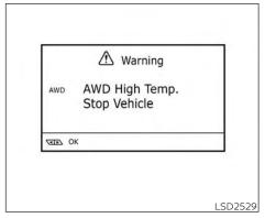
The AWD high temperature message may be displayed while trying to free a stuck vehicle due to increased oil temperature. The driving mode may change to 2-wheel drive. If this message is displayed, stop the vehicle with the engine idling, as soon as it is safe to do so. Then if the message turns off, you can continue driving.
