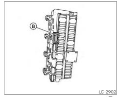
4. Remove the fuse with the fuse puller **B**.
