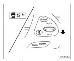
To set cruising speed, accelerate your vehicle to the desired speed, push the SET/switch and release it. The ICC system set indicator (green), vehicle ahead detection indicator, set distance indicator and set vehicle speed indicator (B) will come on. Take vour foot off the accelerator pedal. Your vehicle will maintain the set speed.
