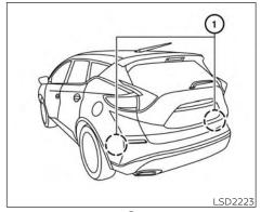
The radar sensors ① can detect an approaching vehicle from up to approximately 66 ft. (20 m) away.
