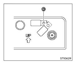
Mark the center of the hole @ on both sides with a felt-tip pen. Remove the bracket from the bumper, and then open 0.9 to 1.0 inch (22 to 25 mm) diameter holes on the bumper using the marks @ as a center.
