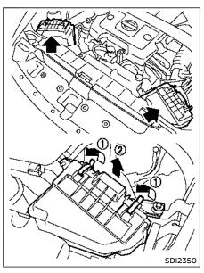
Remove the retainers (i) as illustrated and pull out the filter element 2.
