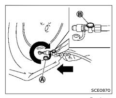
5. Remove the protective cap (a) of the hose and screw the hose securely onto the tire valve. Make sure that the pressure release valve (B) is securely tightened. Make sure that the air compressor switch is in the OFF (○) position, and then insert its power plug into the power outlet in the vehicle.
