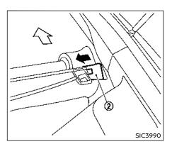
To remove the cargo cover unit, stow the cover and pull the holder ② to the opposite side.
