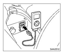
Open the console lid and connect the iPod® cable to the USB connection port. If compatible, the battery of the iPod® is charged while the connection to the vehicle.
