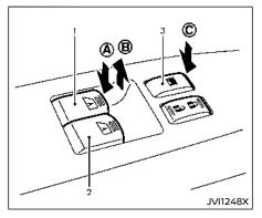
Locking passengers' window When the lock button © is pushed in, only the driver side window can be opened or closed. Push it in again to cancel.
