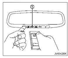
Using both hands, simultaneously press and hold the desired HomeLink® button and handheld transmitter button. DO NOT release until the HomeLink® indicator light ① flashes slowly and then rapidly. When the indicator light flashes rapidly, both buttons may be released. (The rapid flashing indicates successful programming.)
