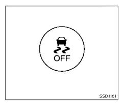
Push the VDC OFF switch again or restart the engine to turn on the system. (See "Vehicle Dynamic Control (VDC) system" (P.5-30).)
