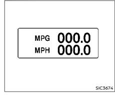
Average fuel consumption (MPG or I (liter)/100 km) and speed (MPH or km/h)
