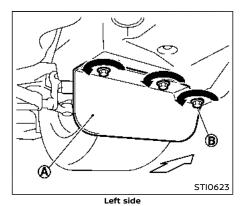
This vehicle is equipped with air deflectors in front of the front wheels. The deflectors will change the air flow to help improve aerodynamic performance.
