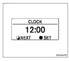
3. Push the switch a for a short time to complete the clock adjustment.
