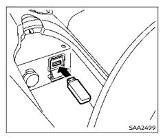
Open the console lid and connect a USB memory as illustrated. Then, push the DISC-AUX button repeatedly to switch to the USB memory mode.
