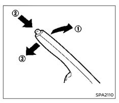
To apply: Pull the parking brake lever up
