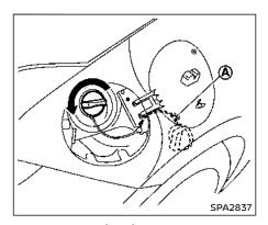
To remove the fuel-filler cap:
