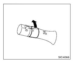
FOG LIGHT SWITCH (if so equipped) To turn on the rear fog light, turn the headlight switch to the position, then turn the fog light switch to the O# position.
