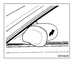
Foldable outside mirrors Fold the outside mirror by pushing it toward the rear of the vehicle.
