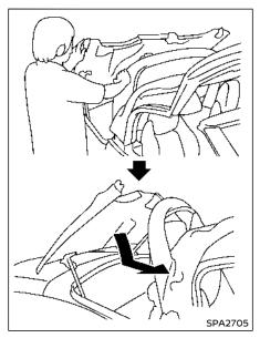
d. Pull down and slide the storage lid to close while holding the rear soft top from the right and left side of the vehicle.
