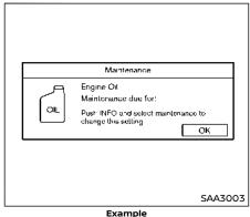
The Reminder will be automatically displayed when the specified distance has been driven and every time the ignition switch is pushed to the ACC or ON position. The reminder will not appear while driving.
