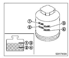
Check the fluid level in the reservoir.
