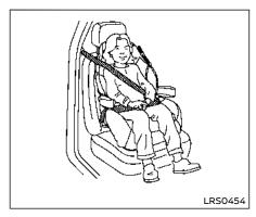
3. The booster seat should be positioned on the vehicle seat so that it is stable. If necessary, adjust or remove the head restraint/headrest to obtain the correct booster seat fit. If the head restraint/headrest is removed, store it in a secure place. Be sure to reinstall the head restraint/headrest when the booster seat is removed. See "Head restraints/headrests" (P.1-6) for head restraint adjustment, removal and installation information.
