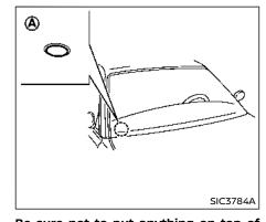
Be sure not to put anything on top of the photo sensor (A) located on the top of the instrument panel. The photo sensor controls the autolight; if it is covered, the photo sensor reacts as if it is dark and the headlights will illuminate.
