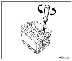
Remove the battery vent caps with a screwdriver as shown.
