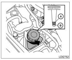
Check the fluid level in the reservoir.
