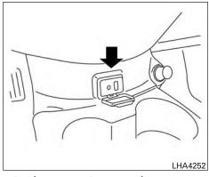
USB (Universal Serial Bus) **CONNECTION PORT (models** without Navigation System) (if so equipped)
