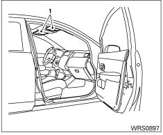
SRS Air Bag Warning Labels (located on the sun visors)
