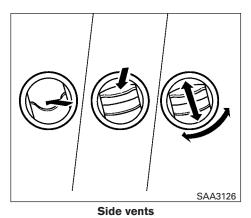
Adjust the air flow direction of the vents by opening, closing or rotating.
