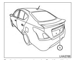
To display the rear view, the RearView Monitor system uses a camera located next to the trunk handle 1.
