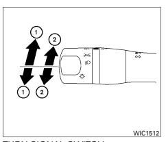
latch, and release the lever. The turn signal will automatically flash three times. Choose the appropriate method to signal a lane change based on road and traffic conditions.
