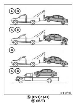
NISSAN recommends that your vehicle be towed with the driving (front) wheels off the ground or place the vehicle on a flat bed truck as illustrated.
