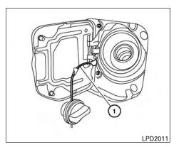
To remove the fuel-filler cap:
