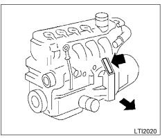
**HR16DE** engine **ENGINE SERIAL NUMBER**
