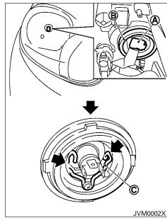
Replacing the halogen headlight bulb
