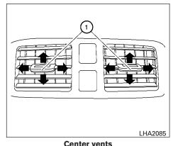
Adjust the air flow direction of the vents by moving the slide as indicated (1).
