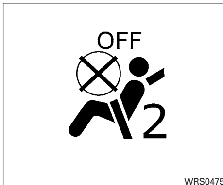
Front passenger air bag and status light
