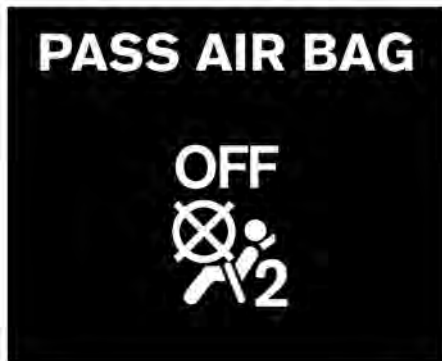
Front passenger air bag status light
