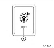
The warning systems switch is used to turn on and off the Blind Spot Warning (BSW) system that is activated using the settings menu on the vehicle information display.
