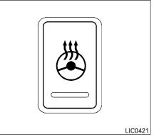
The heated steering wheel system is designed to operate only when the surface temperature of the steering wheel is below approximately 68°F (20°C).
