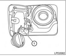
To remove the fuel-filler cap:
