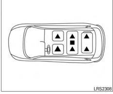
The illustration shows the seating positions equipped with head restraints/headrests.
