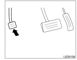
To engage: Firmly depress the parking brake.
