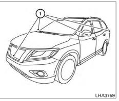
To display the multiple views, the Around View® Monitor system uses cameras located in the front grille, on the vehicle's outside mirrors and one just above the vehicle's license plate (1).
