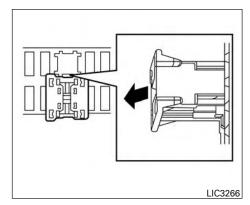
The extended storage switch is used when shipping the vehicle. It is located in the fuse panel to the left of the steering wheel on the instrument panel. If any electrical equipment does not operate, ensure the extended storage switch is pushed fully in place, as shown. STORAGE
