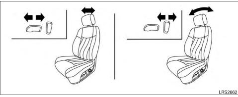
belt fit. For additional information, refer to "Precautions on seat belt usage" in this section. Also, the seatback can be reclined to allow occupants to rest when the vehicle is stopped and the shift lever is in P (Park).
