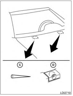
If you wax the surface of the hood, be careful not to let wax get into the washer nozzle O. This may cause clogging or improper windshield-washer operation. If wax gets into the nozzle, remove it with a needle or small pin C.
