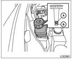
Check the fluid level in the reservoir.
