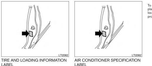
The cold tire pressure is shown on the Tire and Loading Information Label. The label is located as shown.
