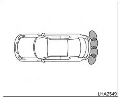
The Camera Aiding Sonar (parking sensor) sounds a tone to inform the driver of obstacles near the bumper.
