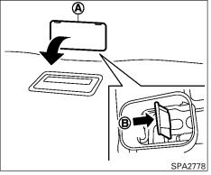
Manual liftgate release (if so equipped)
