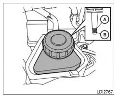
Check the fluid level in the reservoir.
