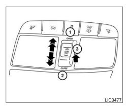
The moonroof will only operate when the ignition switch is placed in the ON position. The moonroof is operational for a period of time, even if the ignition switch is placed in the ACC (if so equipped) or OFF position. If the driver's door or the front passenger's door is opened during this period of time, the power to the moonroof is canceled.
