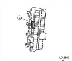
4. Remove the fuse with the fuse puller (B).
