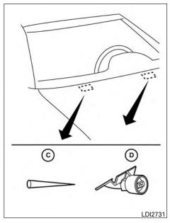
If you wax the surface of the hood, be careful not to let wax get into the washer nozzle **①**. This may cause clogging or improper windshield-washer operation. If wax gets into the nozzle, remove it with a needle or small pin C.
