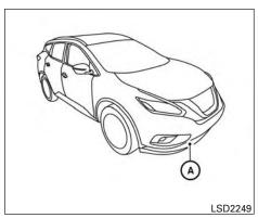
The PFCW system uses a radar sensor (A) located behind the lower grille of the front bumper to measure the distance to the vehicle ahead in the same lane.
