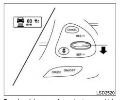
To set cruising speed: accelerate your vehicle to the desired speed, push the SET/- switch and release it. The ICC system set indicator (green), vehicle ahead detection indicator, set distance indicator and set vehicle speed indicator (B) will come on. Take your foot off the accelerator pedal. Your vehicle will maintain the set speed.
