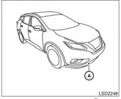
The FEB system uses a radar sensor (A) located on the front of the vehicle to measure the distance to the vehicle ahead in the same lane.
