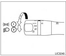
Type A (if so equipped) HEADLIGHT CONTROL SWITCH
