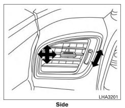
Adjust air flow direction by moving the vent slides.
