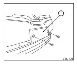
To mount the front license plate, attach the license plate bracket 1 to the plastic finisher at the location marks (small dimples) using the two 6 mm screws provided.
