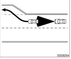
When driving on the freeway at a set speed and approaching a slower traveling vehicle ahead, the ICC system will adjust the speed to maintain the distance, selected by the driver, from the vehicle ahead. If the vehicle ahead changes lanes or exits the freeway, the ICC system will accelerate and maintain the speed up to the set speed. Pay attention to the driving operation to maintain control of the vehicle as it accelerates to the set speed.
