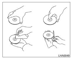
A new disc may be rough on the inner and outer edges. Remove the rough edges by rubbing the inner and outer edges with the side of a pen or pencil as illustrated.
