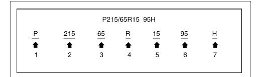
7. H: Tire speed rating. You should not drive the vehicle faster than the tire speed rating.
