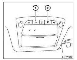
When the ON switch (1) is pressed, the footwell lights (if so equipped), step lights (if so equipped), map lights and rear personal lights will automatically turn on and stay on for a period of time when:
