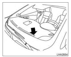
The sunload sensor, located on the driver's side of the instrument panel, helps the system maintain a constant temperature. Do not put anything on or around this sensor.
