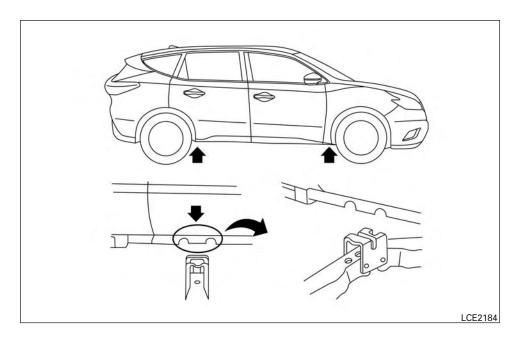
Jacking up vehicle and removing the damaged tire
