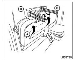
1. To access the jump seat extension (passenger's side only) (A) on the jump seat, pull up (B) on the extension to unfold it to the open position. Then unfold the two support leas © and lower the jump seat to the full open seating position.
