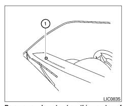
Be sure you do not put anything on top of the autolight sensor (1) located in the top side of the instrument panel. The autolight sensor controls the autolight: if it is covered, the autolight sensor reacts as if it is dark out and the headlights will illuminate. If this occurs while parked with the engine off and the switch in the ON position, your vehicle's battery could become discharged.
