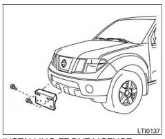
INSTALLING FRONT LICENSE PLATE WITH GROMMETS
