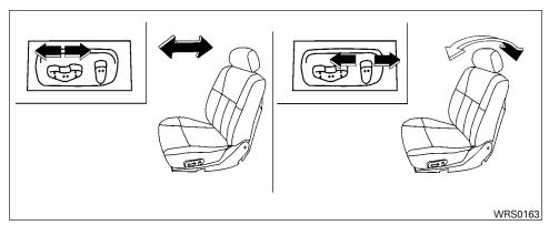
The reclining feature allows adjustment of the seatback for occupants of different sizes for added comfort and to help obtain proper seat belt fit. For additional information, refer to "Precautions on seat belt usage" in this section. Also, the seatback can be reclined to allow occupants to rest when the vehicle is stopped and the shift lever is in P (Park) or N (Neutral) position with the parking brake fully applied.
