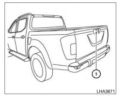
To display the rear view, the RearView Monitor system uses a camera located next to the liftgate handle (1).
