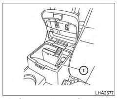
USB (Universal Serial Bus) CONNECTION PORT (models with Navigation System)
