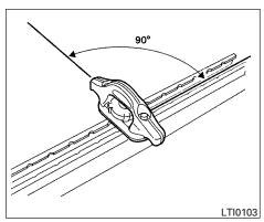
3. Insert the cleat into the channel perpendicular to the channel as shown. Then rotate the cleat clockwise 90° and slide it to the desired location.
