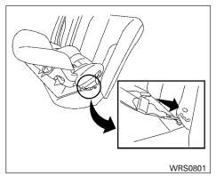
Rear-facing webbing-mounted - step 4 4. Secure the child restraint anchor attach-
