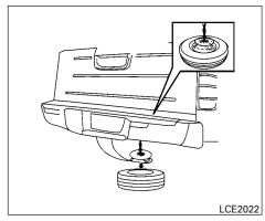
3. To reinstall the wheel, insert the tire chain through the wheel. Be sure the rubber spacer is centered on the wheel before lifting. Use the assembled jack rod and slowly rotate the winch clockwise to raise the wheel to the vehicle.
