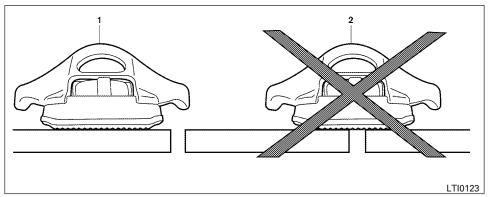
1 correct installation, 2 incorrect installation
