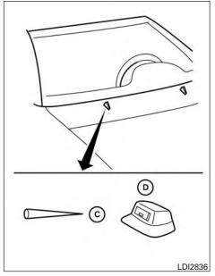
Be careful not to let anything get into the washer nozzle (D). This may cause clogging or improper windshield-washer operation. If something gets into the nozzle, remove it with a needle or small pin (C).
