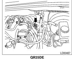
CHECKING ENGINE OIL LEVEL
