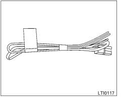
To install the electric trailer brake controller jumper harness, perform the following procedure:
