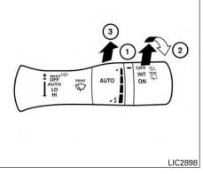
If the rear window wiper operation is interrupted by snow, etc., the wiper may stop moving to protect its motor. If this occurs, turn the wiper switch to OFF and remove the snow, etc. on and around the wiper arms. After about 1 minute, turn the switch ON again to operate the wiper.
