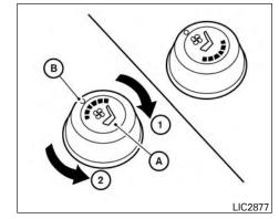
The climate controlled seat warms up or cools down the front seat by blowing warm or cool air from under the surface of the seat. The climate control switch is located on the center console.
