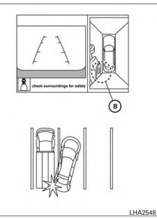
There may be a small distance visible between the vehicle and the object in the bird-eye view on the display (B).
