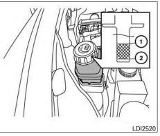
Check the fluid level in the reservoir.
