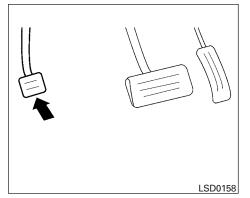
To engage: Firmly depress the parking brake.
