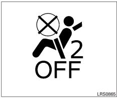
7. If the booster seat is installed in the front passenger seat, place the ignition switch in the ON position. The front passenger air bag status light and may or may not illuminate, depending on the size of the child and the type of booster seat being used. For additional information, refer to "Front passenger air bag and status light" in this section.
