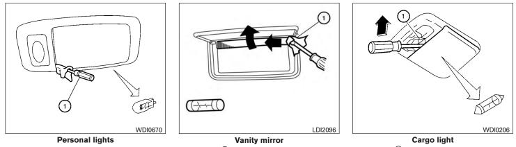
Use a cloth to protect the housing and suitable tool 1 to remove lens.
