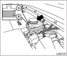
Check the fluid level in the reservoir. If the brake fluid is below the MIN line (B), the brake warning light will illuminate. Add brake fluid up to the MAX line (A). For additional information, refer to "Recommended fluids/lubricants and capacities" in the "Technical and consumer information" section of this manual for the recommended type of brake fluid.
