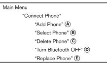
Use the Connect Phone commands to manage the phones connecting to the vehicle or to enable the Bluetooth® function on the vehicle.
