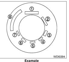
Federal law requires tire manufacturers to place standardized information on the sidewall of all tires. This information identifies and describes the fundamental characteristics of the tire and also provides the tire identification number (TIN) for safety standard certification. The TIN can be used to identify the tire in case of a recall.
