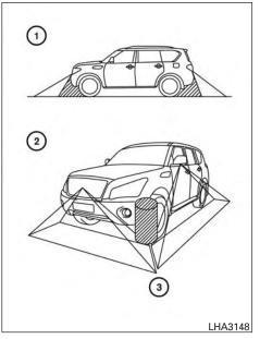
There are some areas where the system will not show objects and the system does not warn of moving objects. When in the front or rear view display, an object below the bumper or on the ground may not be viewed ①. When in the bird's-eye view, a tall object near the seam (3) of the camera viewing areas will not appear in the monitor (2).
