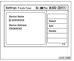
6. The Device Name and Device Address are displayed on the screen. Select the "Select" key to make this device the active Bluetooth® audio player. Select the "Edit" key to edit the details of the player, such as Device Name. Select the "Delete" key to delete the device.
