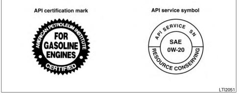
Committee (ILSAC) certification and SAE viscosity standard. These oils have the API certification mark on the front of the container. Oils which do not have the specified quality label should not be used as they could cause engine damage.
