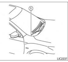
Be sure you do not put anything on top of the autolight sensor located in the top side of the instrument panel (1). The autolight sensor controls the autolight; if it is covered, the autolight sensor reacts as if it is dark out and the headlights will illuminate. If this occurs while parked with the engine off and the ignition switch placed in the ON position, your vehicle's battery could become discharged.
