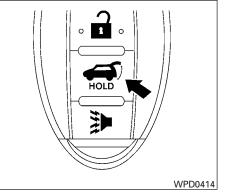
Releasing the rear liftgate (if so equipped)
