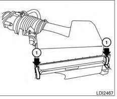
Clean and replace the air cleaner filter according to the maintenance log shown in the "NISSAN Service and Maintenance Guide". When replacing the filter, wipe the inside of the air cleaner filter housing and the cover with a damp cloth.
