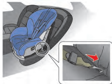
Forward-facing web-mounted — step 2
