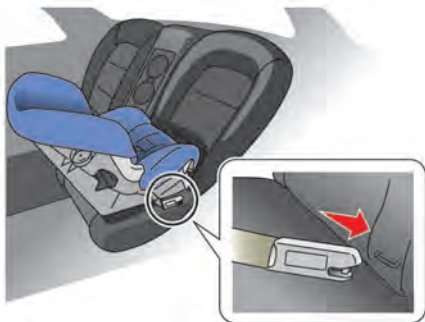
Rear-facing rigid-mounted — step 2
