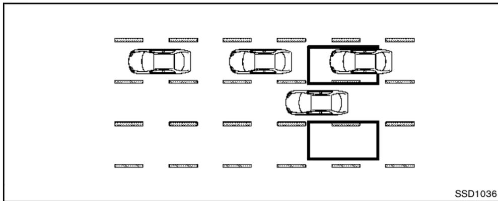
If the driver activates the turn signal while another vehicle is in the detection zone, then the BSW indicator light flashes and a chime will sound twice.
