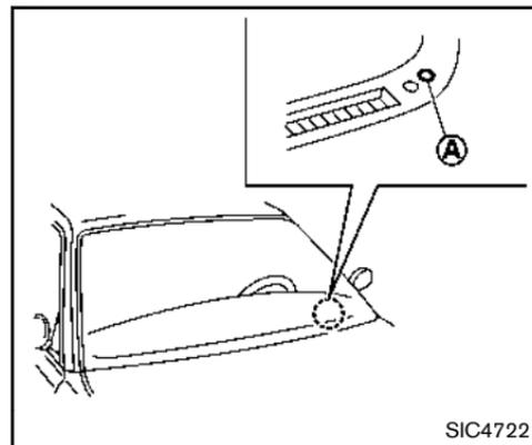
**Be sure not to put anything on top of the photo sensor
