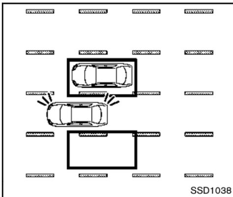
If the driver activates the turn signal, then the BSW indicator light flashes and a chime will sound twice.
