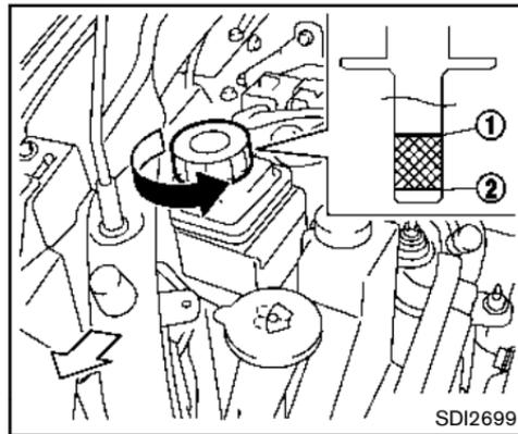
Check the fluid level in the reservoir.
