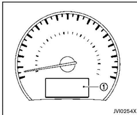
The dot matrix liquid crystal display
