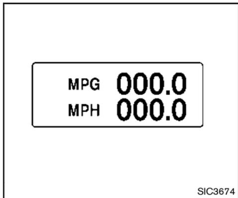
Average fuel consumption (MPG, l/100 km or km/l) and speed (MPH or km/h)
