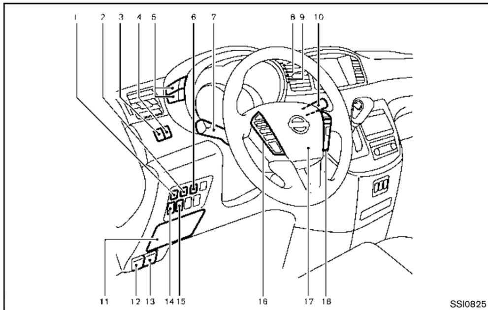
1. Vehicle Dynamic Control (VDC) OFF switch
