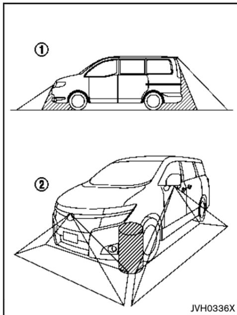
There are some areas where the system will not show objects. When in the front or the rear view display, an object below the bumper or on the ground may not be viewed ①. When in the bird's-eye view, a tall object near the seam of the camera viewing areas will not appear in the monitor ②.
