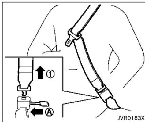
tongue ① may also be released. Release the connector tongue by inserting a suitable tool (such as a key) into the connector buckle A. If the seat belt cannot be unbuckled or is already unbuckled, release the child by cutting the seat belt with a suitable tool (such as a knife or scissors) to release the seat belt.
