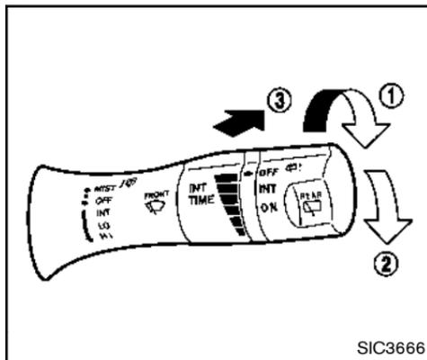
The rear window wiper and washer operate when the ignition switch is in the ON position. Turn the switch clockwise from the OFF position to operate the wiper.
