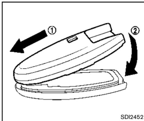
4. Align the tips of the upper and lower parts ①, and then push them together ② until it is securely closed.
