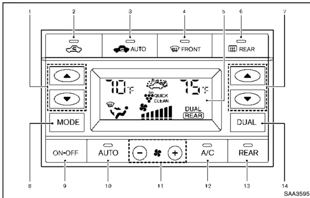
9. "ON-OFF" button for air conditioning system
