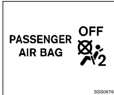
7. If the booster seat is installed in the front passenger seat, push the ignition switch to the ON position. The front passenger air bag status light
