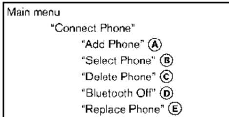
Use the Connect Phone commands to manage the phones connecting to the vehicle or to enable the Bluetooth<sup>®</sup> function on the vehicle.
