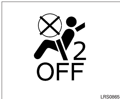
Front passenger air bag and status light
