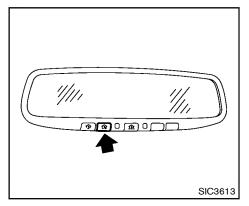
Using both hands, simultaneously push and hold both the HomeLink® button you want to program and the hand-held transmitter button.
