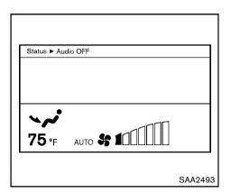
For the models with navigation system, push the "STATUS" button to display the heater and air conditioner status screen. (See "How to use STATUS button" (P.4-7).)
