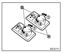
The climate controlled seat warms up or cools down the front seats by blowing warm or cool air from the surface of the seat. The switches located on the center console can be operated independently of each other.
