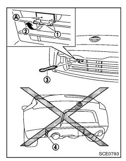
1. Access the mounting hole for the recovery hook.
