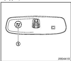
The Type A system does not have an IV ① on the back of the mirror. Move the mirror to see if the IV is present. If the IV is **not** on the mirror, use the procedure in this section to program the HomeLink® Universal Tranceiver. If the IV is on the mirror, see "HomeLink® Universal Transceiver (Type B)" (P.2-54).
