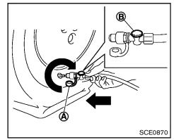
Remove the protective cap (A) of the hose and screw the hose securely onto the tire valve. Make sure that the pressure release valve (B) is securely tightened. Make sure that the air compressor switch is in the OFF ( ) position, and then insert its power plug into the power outlet in the vehicle.
