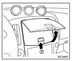
INSTRUMENT POCKET (except for navigation system equipped models) To open the lid, push the knob up (1). To close, push the lid down.
