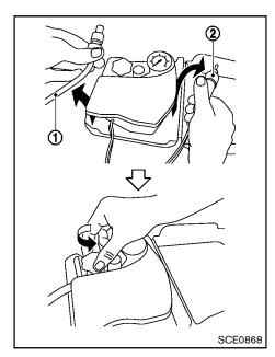
2. Take the hose (1) and the power plug (2) out of the air compressor. Remove the cap of the bottle holder from the air compressor.
