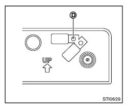
Mark the center of the hole (D) on both sides with a felt-tip pen. Remove the bracket from the bumper, and then open 0.9 to 1.0 inch (22 to 25 mm) diameter holes on the bumper using the marks (D) as a center.
