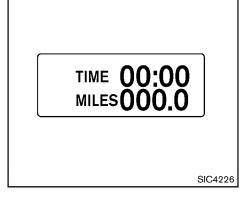
Elapsed time and trip odometer (MILES or km)
