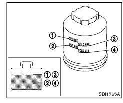
Check the fluid level in the reservoir.
