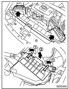
Remove the retainers ① as illustrated and pull out the filter element ②.
