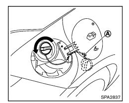
To remove the fuel-filler cap:
