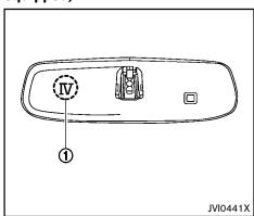
The Type B system can be identified by the IV ① on the back of the mirror. Move the mirror to see if the IV is present. If the IV is on the mirror, use the procedure in this section to program the HomeLink® Universal Transceiver. Otherwise, use the procedure in "HOMELINK® UNIVERSAL TRANSCEIVER (Type A) (if so equipped).
