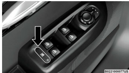
Window Lockout Switch
