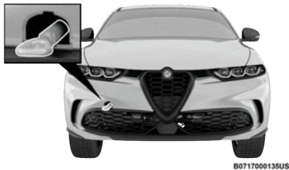
Front Tow Eye Installed
