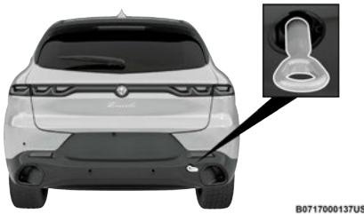
Rear Tow Eye Installed
