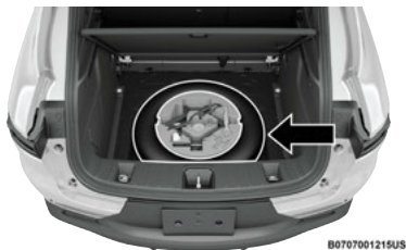
Damaged Tire Stowage
