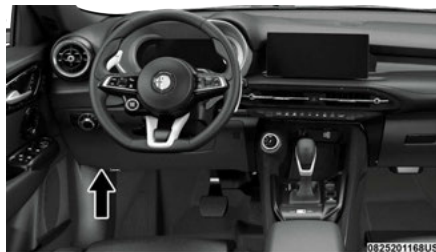
Interior Fuse Box Location
