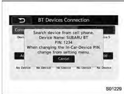
When the “Add” key is selected (Waiting for the connection request from a device).
