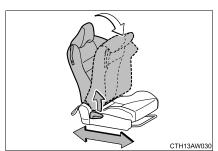
Lift the seatback angle adjustment lever.
