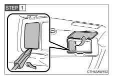
Open the cover and remove the lens.
