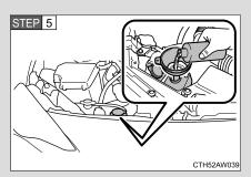
Add engine coolant if necessary.
