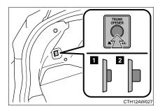
Turn the main switch in the trunk lid off to disable the trunk lid opener.
