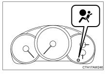
A diagnostic system continually monitors the readiness of the SRS airbag system (including front seatbelt pretensioners) while the vehicle is being driven. The SRS airbag system warning light will show normal system operation by illuminating for approximately 6 seconds when the ignition switch is turned to the "ON" position.
