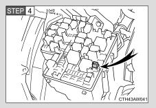
Remove the fuse with the pullout tool.
