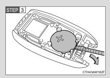
Remove the depleted battery.
