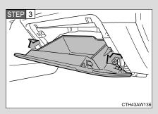
Push in each side of the glove box and pull the glove box toward you to disconnect the claws.
