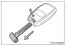
To take out the mechanical key, push the release knob and take the key out.
