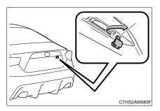
Turn the mechanical key clockwise to open.
