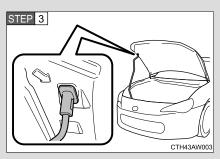
Hold the engine hood open by inserting the supporting rod into the slot.
