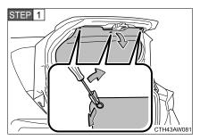
Remove the trunk lid panel cover clips and partly remove the trunk lid panel cover.
