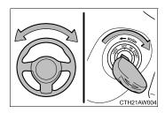
When starting the engine, the engine switch may seem stuck in the "LOCK" position. To free it, turn the key while turning the steering wheel slightly left and right.
