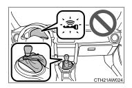
Vehicles with an automatic transmission: Check that the select lever is securely set in P. The engine may not start if the select lever is displaced out of P. The keyless access with push button start system indicator light (green) will flash quickly.
