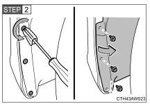
Remove the clips and partly remove the fender liner.
