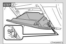
Open the glove box. Slide off the damper.
