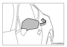
Push the mirror back in the direction of the vehicle's rear.
