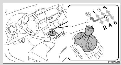
Fully depress the clutch pedal before operating the shift lever, and then release it slowly.
