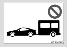
Your vehicle is not designed to be dinghy towed behind a motor home or other vehicle with the wheels (2 or 4) on the ground. Serious damage can result.
