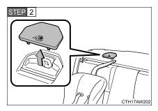
Remove the anchor bracket cover.
