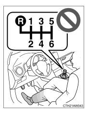
Do not shift the shift lever without depressing the clutch pedal.
