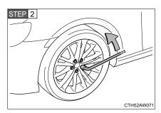
Slightly loosen the wheel nuts (one turn).
