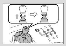
Shift the shift lever to R while lifting up the ring section.
