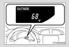
The outside temperature display can be switched by pressing the "DISP" switch.  $(\rightarrow P. 198)$
