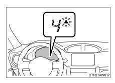
To help enable fuel-efficient driving, the shift-up indicator flashes 3 times to indicate upshift timing.
