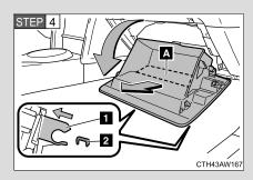
Lower the glove box slowly until surface \( \bar{\textstyle }\) is horizontal with the floor, then pull it out. (Simply pulling with gentle force will disengage the lower claws.)
