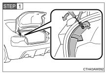
Remove a clip and partly remove the cover.
