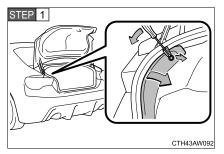
Remove a clip and partly remove the cover.
