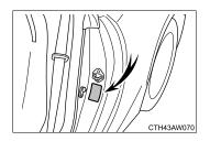
For the GAWR, see the Certification Label. For the maximum load of the tire, see the load limit at maximum cold tire inflation pressure mentioned on the sidewall of the tire.  $(\rightarrow P. 430)$
