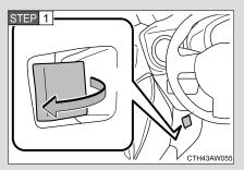
Pull the engine hood release lever.
