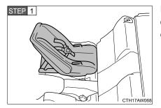
Place the child restraint system on the rear seat facing the rear of the vehicle.
