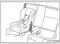
Seatbelts equipped with a child restraint locking mechanism (ALR/ELR belts except driver's seatbelt) (→P. 58)
