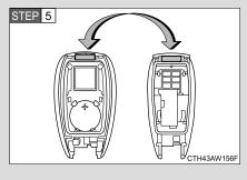
Align the protruding part with the slot and install the cover.
