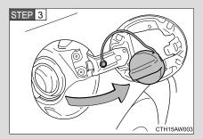
Hang the fuel tank cap on the back of the fuel filler lid.
