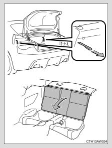
Pull the both left and right seatback lock release straps in the trunk lid to fold down the seatback.
