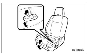
To adjust the seat cushion angle, pull up or push down the front end of the control switch.
