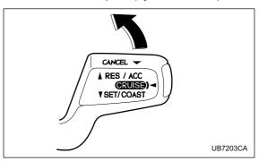
Push the control lever upward in the "RES/ACC" direction and hold it until the vehicle reaches the desired speed. Then, release the control lever. The vehicle speed at that moment will be memorized and treated as the new set speed.
