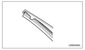
Securely lock the end of the plastic support as shown in the illustration. If the rubber is not retained properly, the wiper may scratch the rear window glass.
