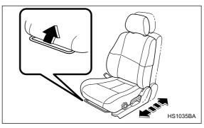
Pull the lever upward and slide the seat to the desired position. Then release the lever and move the seat back and forth to make sure that it is securely locked into place.
