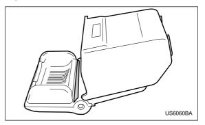
Particles of ash and tobacco will accumulate around the hinges of the ashtray's inner lid. Clean them off using a toothbrush or other narrow-ended implement.
