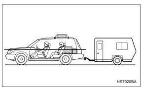
Owing to the self-leveling suspension, the vehicle body is adjusted to the proper position after several drive trips, even if the rear of the vehicle is lowered by loaded cargos or a coupled trailer.
