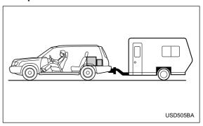
Vehicle capacity weight of the vehicle is 900 lbs (408 kg), which is indicated on the vehicle placard with the statement "The combined weight of occupants and cargo should never exceed 408 kg or 900 lbs".
