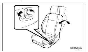
To adjust the angle of the seatback, move the control switch forward or backward
