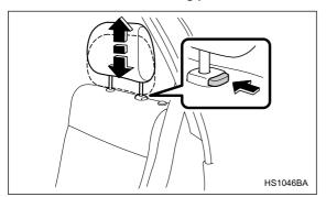
To raise the head restraint, pull it up. To lower it, push the head restraint down while depressing the release button on the top of the seatback.
