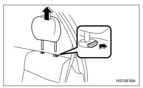
1. Remove the head restraint at the seating position where the child restraint system has been installed with the lower anchorages or seatbelt; lift up the head restraint while pressing the release button. Store the head restraint in the cargo area. Avoid placing the head restraint in the passenger compartment to prevent it from being thrown around in the passenger compartment in a sudden stop or a sharp turn.
