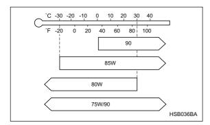
SAE viscosity No. and applicable temperature
