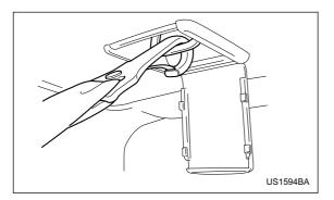
8. If the child restraint system requires a top tether, latch the hook onto the top tether anchor and tighten the top tether. See the "Top tether anchorages" for additional instructions.
