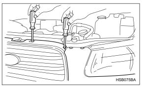
1. Remove the front grille. Use a screwdriver to detach the four clips at the top and the three hooks on the left, right and center.
