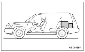
Vehicle capacity weight of the vehicle is 900 lbs
