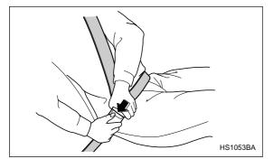
Push the button on the buckle. Before closing the door, make sure that the belts are retracted properly to avoid catching the belt webbing in the door.
