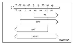
SAE viscosity No. and applicable temperature
