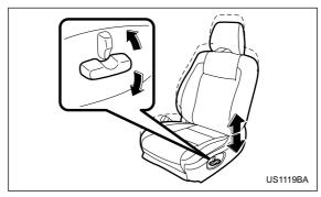
To adjust the seat height, pull up or push down the rear end of the control switch.
