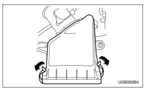
1. Unsnap the two clamps holding the air cleaner case cover.
