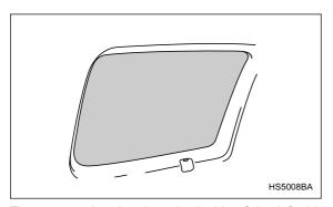
The antenna is printed on the inside of the left side rear quarter window glass.
