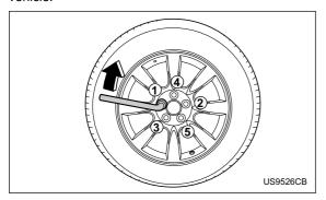
13.Use the wheel nut wrench to securely tighten the wheel nuts to the specified torque, following the tightening order in the illustration.
