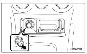
The cigarette lighter operates only when the ignition switch is in the "ON" and "ACC" positions.
