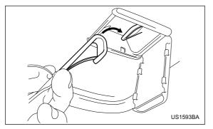
2. Open the cover flaps to use the anchorages. Fasten the top tether hook of the child restraint system to the appropriate top tether anchorage.
