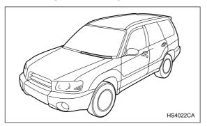
Always keep the front ventilation inlet grille free of snow, leaves, or other obstructions to ensure efficient heating and defrosting. Since the condenser is located in front of the radiator, this area should be kept clean because cooling performance is impaired by any accumulation of insects and leaves on the condenser
