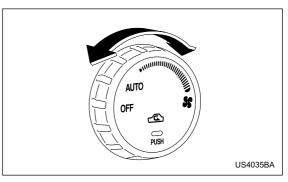
The fan operates only with the ignition switch in the ON position. The fan speed control dial is used to select the AUTO (automatic control) mode or to select the desired fan speed. The dial's positions and their functions are as follows:
