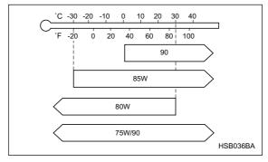
SAE viscosity No. and applicable temperature
