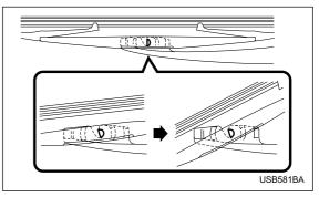
2. Turn the wiper blade assembly counterclockwise.
