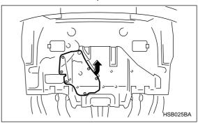
4. Open the access cover by removing the six clips and turning the access cover counterclockwise. The drain plug will be exposed.
