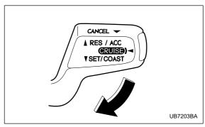
Push the control lever downward in the "SET/COAST" direction and hold it until the vehicle reaches the desired speed. Then, release the control lever. The vehicle speed at that moment will be memorized and treated as the new set speed.
