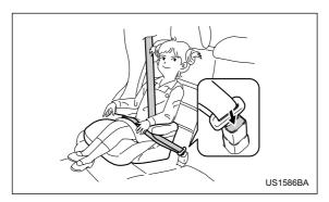
4. To remove the booster seat, press the release button on the seatbelt buckle and allow the belt to retract.
