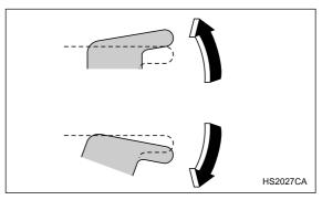
To open the passengers' windows, push the appropriate switch down and hold it until the window reaches the desired position.
