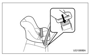
8. To remove the child restraint system, press the release button on the seatbelt buckle and allow the belt to retract completely. The belt will return to the ELR mode.
