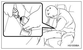
4. After confirming that the webbing is not twisted, insert the connector (tongue) attached at the webbing end into the buckle on the right hand side until a click is heard.
