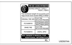
The vehicle placard shows original tire size, recommended cold tire inflation pressure on each tire at maximum loaded vehicle weight, seating capacity and loading information.
