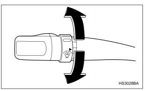
When the headlight switch is in the " <code>=Doa=</code> " or " <code>=Doa=</code> " or " <code>=Doa=</code> " position, you can adjust brightness of the instrument panel illumination for better visibility.
