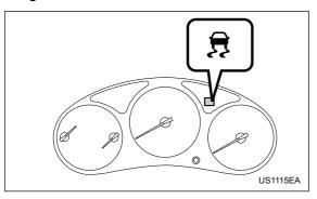
The indicator light turns on when the ignition key is turned to the ON position; it turns off approximately two seconds later. This indicator light flashes during activation of the skid suppression function and is illuminated steadily during activation of the traction control function.
