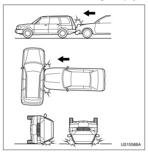
The SRS frontal airbag is basically not designed to deploy if the vehicle is struck from side or from behind, or if it rolls onto its side or roof, or if it is involved in a low-speed frontal collision.
