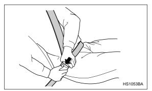
Push the button on the buckle. Before closing the door, make sure that the belts are retracted properly to avoid catching the belt webbing in the door.
