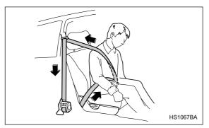
The driver's and front passenger's seatbelts have a seatbelt pretensioner. The seatbelt pretensioners are designed to be activated in the event of an accident involving a moderate to severe frontal collision. Also, the seatbelt pretensioners are designed to be activated in the event of an accident involving a moderate to severe side impact collision.
