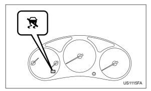
This single light has the function of indicating malfunctions in the Vehicle Dynamics Control system and the function of indicating that the Vehicle Dynamics Con-
