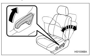
Pull the reclining lever up and adjust the seatback to the desired position. Then release the lever and make sure the seatback is securely locked into place. The seatback placed in a reclined position can spring back upward with force when released. When operating the reclining lever to return the seatback, hold it lightly so that it may be raised back gradually.
