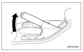
Check the parking brake stroke according to the maintenance schedule in the "Warranty and Maintenance Booklet". When the parking brake is properly adjusted, braking power is fully applied by pulling the lever up seven to eight notches gently but firmly (about 44 lbs, 196 N, 20 kg). If the parking brake lever stroke is not within the specified range, have the brake system checked and adjusted at your SUBARU dealer.
