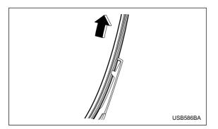
5. Pull the blade rubber assembly out of the plastic support.
