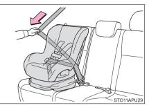
5 While pushing the child restraint system into the rear seat, allow the shoulder belt to retract until the child restraint system is securely in place.
