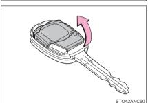
3 Open the case cover and remove the depleted battery.
