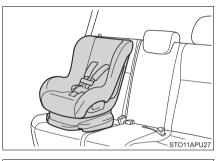
3 Run the seat belt through the child restraint system and insert the plate into the buckle. Make sure that the belt is not twisted.
