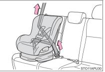
6 If the child restraint has a top tether strap, the top tether strap should be latched onto the top tether strap anchor. ( $\rightarrow$ P. 63)
