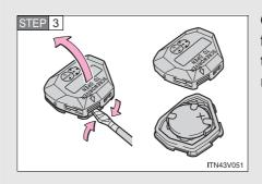
Open the case cover using a flathead screwdriver protected with tape etc. and remove the depleted battery.
