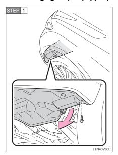
Remove the engine under cover bolt and pull down the engine under cover.
