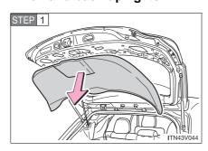
Open the back door and remove the trim board.
