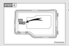
Remove the fuse with the pullout tool.
