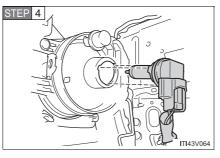
Exchange the light bulb, and install the light bulb.
