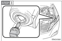
Exchange the light bulb, and install the light bulb.
