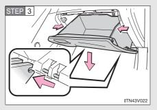
Push each side of the glove box to release the pins. Then disconnect the claws at the bottom and remove the glove box.
