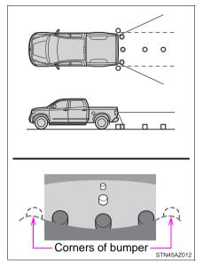
• Items which are located higher than the camera may not be displayed on the monitor.
