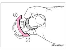
(8) Washer/wiper dual operation Wipers will automatically operate a couple of times after the washer squirts.
