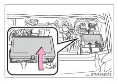
Under the instrument panel Remove the cover.
