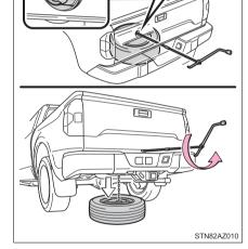
3 After the tire is lowered completely to the ground, remove the holding bracket.
