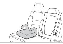
2 Sit the child in the child restraint system. Fit the seat belt to the child restraint system according to the manufacturer's instructions and insert the plate into the buckle. Make sure that the belt is not twisted. STN11A2050
