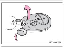
2 Remove the depleted battery.
