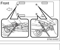
If you use chains or cables to tie down your vehicle, the angles shaded in black must be  $45^{\circ}$ .
