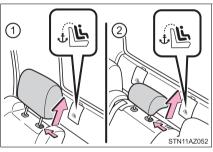
3 Remove the anchor bracket cover.
