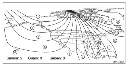
The direction display deviates from the true direction determined by the earth's magnetic field. The amount of deviation varies according to the geographic position of the vehicle.
