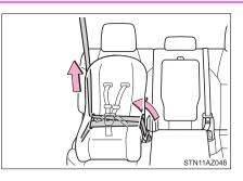
If the child restraint has a top tether strap, the top tether strap should be latched onto the top tether strap anchor.
