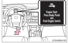
Press the engine switch shortly and firmly.
