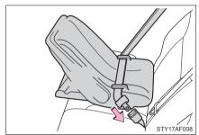
3 Fully extend the shoulder belt and allow it to retract to put it in lock mode. In lock mode, the belt cannot be extended.
