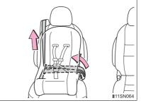
5 If the child restraint has a top tether strap, the top tether strap should be latched onto the top tether strap anchor. ( $\rightarrow$ P. 69, 70)
