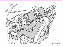
Pre-collision seat belts (front seats of vehicles with pre-collision system)
