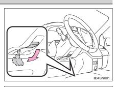
2 Adjust to the ideal position by moving the steering wheel horizontally and vertically.
