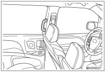
An assist grip installed on the ceiling can be used to support your body while sitting on the seat. An assist grip installed on the pillar can be used when getting in or out of the vehicle and others.
