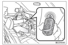
3 Press the engine switch within 10 seconds after the buzzer sounds, keeping the brake pedal depressed.
