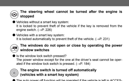
The auto power off function will be operated if the vehicle is left in ACCES-SORY or IGNITION ON mode (the engine is not operating) for a period of time. (→P. 230)
