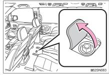
3 Attach the adapter socket over the spare tire clamp bolt.
