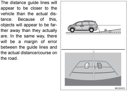
• When the ground behind the vehicle slopes down sharply
