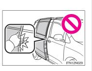
Use caution when using the sliding door closer. The sliding door closer operates even when the power sliding door system is canceled.
