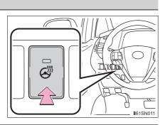
• The heated steering wheel can be used when the engine switch is in IGNI-TION ON mode.
