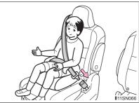
Check that the shoulder belt is correctly positioned over the child's shoulder and that the lap belt is as low as possible. ( $\rightarrow$ P. 28)
