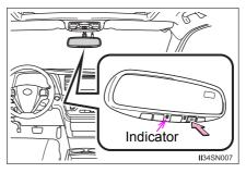
Pressing the button turns the function to off mode. (The indicator also turns off.)
