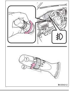
Fog lights can be used when The headlights are on in low beam.
