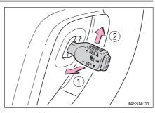
Resuming is available when the vehicle speed is more than approximately 25 mph (40 km/h).
