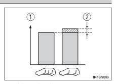
If removing the second seats, it is possible to load extra cargo equal to the weight of the removed seats.
