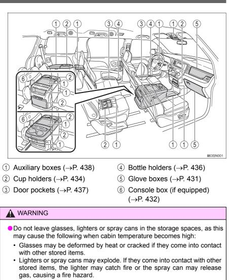
When driving or when the storage compartments are not in use, keep the lids closed.
