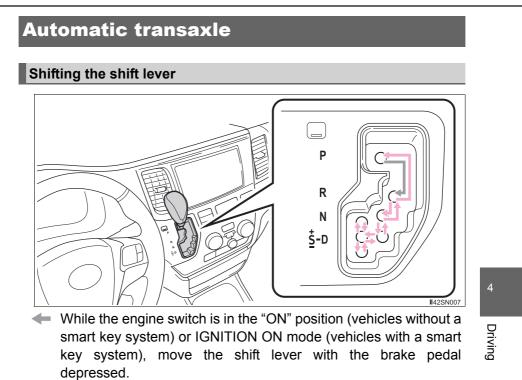
When shifting the shift lever between P and D, make sure that the vehicle is completely stopped.
