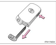
After using the mechanical key, store it in the electronic key. Carry the mechanical key together with the electronic key. If the electronic key battery is depleted or the entry function does not operate properly, you will need the mechanical key. ( $\rightarrow$ P. 588)
