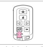
Pressing the switch again while the power back door is operating will cause the operation to reverse. However, the reverse operation cannot be performed for the first second after automatic operation starts, even if the wireless remote control switch is pressed again.
