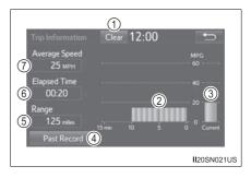
Average fuel consumption for the past 15 minutes is divided by color into past averages and averages attained since the engine switch was last turned to the "ON" position (vehicles without a smart key system) or IGNITION ON mode (vehicles with a smart key system). Use the displayed average fuel consumption as a reference.
