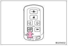
Pressing the switch again while the power back door is operating will cause the operation to reverse. However, the reverse operation cannot be performed for the first second after automatic operation starts, even if the wireless remote control switch is pressed again.
