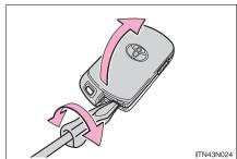
Remove the depleted battery.
