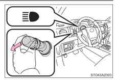
2 Press the Automatic High Beam switch.
