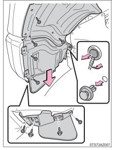
2 Open the fender liner and turn the bulb base counter-clockwise.
