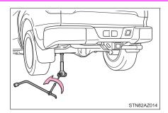
4 Firmly tighten each nut two or three times in the order shown in the illustration.
