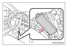
Remove the fuse with the pullout tool.
