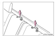
Route the top tether strap through the anchor strap router as shown in the illustration.
