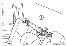
5 Latch the hook onto the anchor strap ring and tighten the top tether strap.
