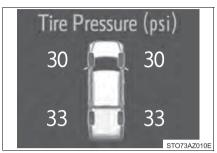
• If the tire pressure drops below a predetermined level, the driver is warned by a screen display and a warning light.
