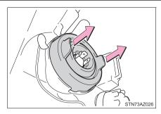
4 Release the bulb retaining spring.
