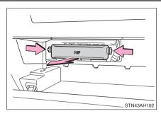
6 Pull the filter out of the filter outlet.
