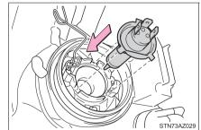
7 Install the bulb retaining spring.
