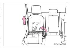
5 If the child restraint has a top tether strap, the top tether strap should be latched onto the top tether strap anchor. (→P. 67, 70)
