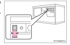
Press and hold the desired HomeLink® button (inside the vehicle) for 2 seconds and release it. Repeat this sequence (press/hold/release) up to 3 times to complete programming.
