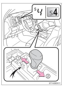
The initial shift range in S mode is set automatically to 5 or 4 according to vehicle speed. However, the initial shift range may be set to 3 if the AI-SHIFT has operated while the shift lever was in the D position. ( $\rightarrow$ P. 200)
