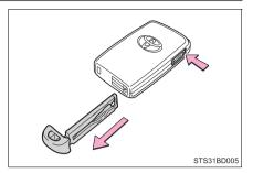
After using the mechanical key, store it in the electronic key. Carry the mechanical key together with the electronic key. If the electronic key battery is depleted or the entry function does not operate properly, you will need the mechanical key. ( $\rightarrow$ P. 557)
