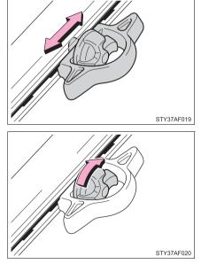
5 Check the tie-down cleat to confirm that it is locked into a detent and securely mounted to the deck rail system.
