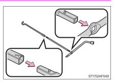
2 Insert the end of the jack handle extension into the lowering screw and turn it counterclockwise.
