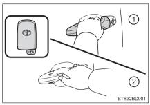
2 Touch the lock sensor (the indentation on the upper part or lower part of the driver's door handle) to lock the doors.
