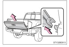
3 Slide the tailgate a little to the right to unhook the left side being mindful of tailgate righthand side clearance to vehicle's rear bumper.
