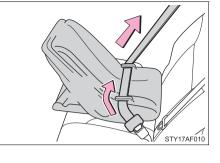
4 While pushing the child restraint system into the rear seat, allow the shoulder belt to retract until the child restraint system is securely in place.
