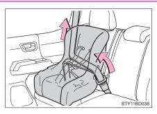
5 If the child restraint has a top tether strap, the top tether strap should be latched onto the top tether strap anchor. ( $\rightarrow$ P. 63, 65)
