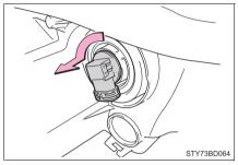
3 Set the new light bulb. Align the 3 tabs on the light bulb with the mounting and insert.
