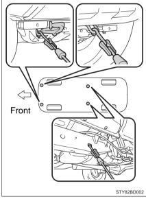
If you use chains or cables to tie down your vehicle, the angles shaded in black must be  $45^{\circ}$ .
