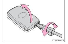
3 Remove the depleted battery.
