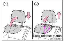
Vertical adjustment (center head restraint)
