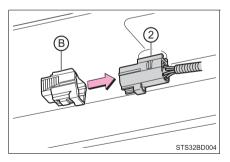
3 Pull out the plastic wire protector located in the vehicle bed by pressing the tabs and pulling the protector.
