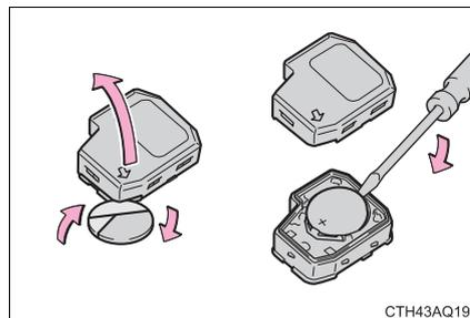
**Replacing the battery (vehicles with a smart key system)**
