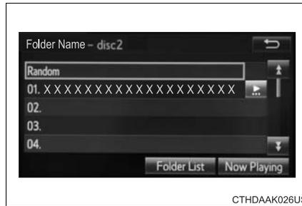
When an MP3/WMA/AAC disc is being used, the folder can be selected. When a Bluetooth® device, USB memory device or iPod is being used, the album can be selected.
