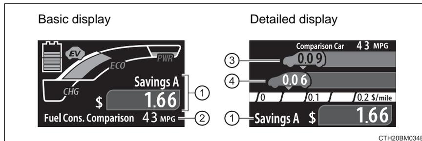
With 2 types of displays available, the cost of the consumed fuel can be displayed or the fuel consumption's comparison can be displayed.
