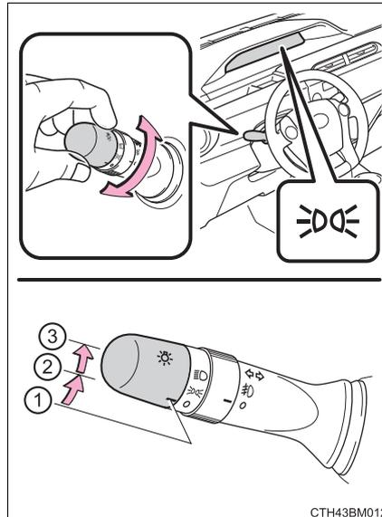
**Turning on the high beam headlights**
