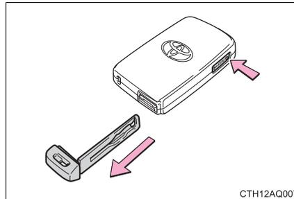
After using the mechanical key, store it in the electronic key. Carry the mechanical key together with the electronic key. If the electronic key battery is depleted or the entry function does not operate properly, you will need the mechanical key. (→P. 516)
