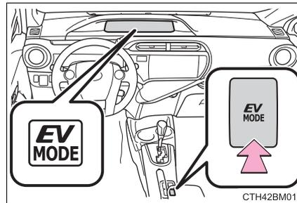
**■ Switching to EV drive mode when the gasoline engine is cold**
