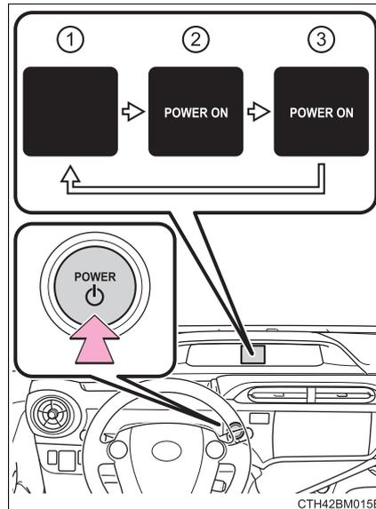
\*: If the shift lever is in a position other than P when turning off the hybrid system, the “POWER” switch will be turned to ACCESSORY mode, not to off.
