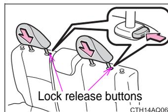
■ **Adjusting the height of the head restraints (vehicles with adjustable type head restraints)**
