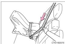
5 While pushing the child restraint system down into the rear seat, allow the shoulder belt to retract until the child restraint system is securely in place.
