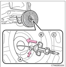
11 Tilt the holding bracket (B) so that it can easily be passed through the wheel opening. After passing the holding bracket through the wheel opening, remove the hoist assembly (C).
