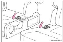
4 Pass the outer seat belts through the seat belt hangers and secure the seat belt plates.
