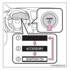
If the hybrid system is stopped with the shift lever in a position other than P, the power switch will not be turned off but instead be turned to ACCESSORY mode. Perform the following procedure to turn the switch off:
