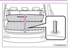
2 To secure the center deck board, remove the hook on the backside of the center deck board and attach the hook to the head restraint on the third seats as shown.
