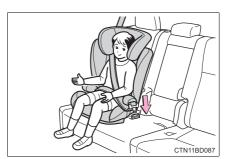
Check that the shoulder belt is correctly positioned over the child's shoulder and that the lap belt is as low as possible.  $(\rightarrow P. 32)$
