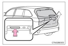
Pressing the switch while the back door is opening/closing stops the operation.
