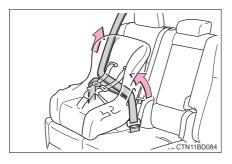
6 If the child restraint has a top tether strap, the top tether strap should be latched onto the top tether strap anchor. (→P. 76)
