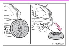
6 When stowing the tire, make sure that the hoist assembly is placed perpendicular to the wheel opening.
