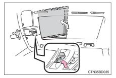
The moon roof can be tilted down only when it is in the tilt-up position.
