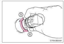
(7) Washer/wiper dual operation Wipers will automatically operate a couple of times after the washer squirts.
