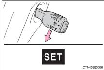
To change the set speed, operate the lever until the desired set speed is displayed.
