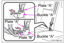
3 Holding plate "A" and "B" together, insert both plates into the holder on the roof.
