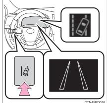
Press the LDA switch to activate the system.
