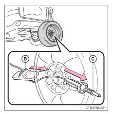
3 Fully depress the secondary latch (A) and install the bracket (B) to the hoist assembly (C).
