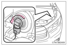
3 Unplug the connector while pressing the lock release.
