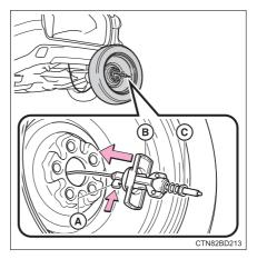
10 Tilt the bracket (B) and pass it through the wheel opening. Then remove the hoist assembly (C).
