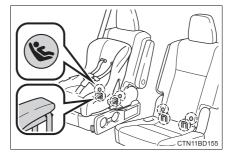
Seat belts equipped with a child restraint locking mechanism (ALR/ELR belts except driver's seat belt) (→P. 36)
