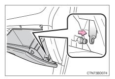
3 Push in each side of the glove box to disconnect the upper claws. Then pull out the glove box and disconnect the lower claws.
