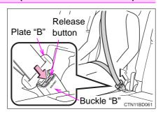
2 To release plate "A", insert the key (→P. 124) or plate "B" into the hole on buckle "A".
