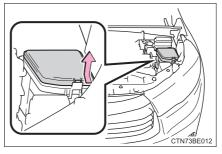
► Engine compartment (type C fuse box)
