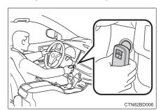
3 Firmly depress the brake pedal.
