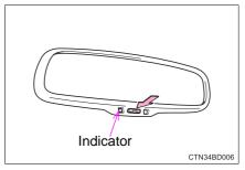
When the automatic anti-glare function is in ON mode, the indicator illuminates.
