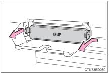
6 Remove the air conditioning filter and replace it with a new one.
