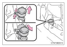
For the left side only: Remove the fuse box.
