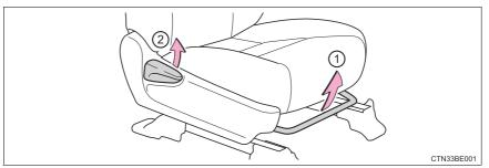
1 Seat position adjustment lever 2 Seatback angle adjustment lever
