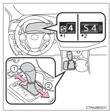
The initial shift range in S mode is set automatically to 5 or 4 according to vehicle speed.
