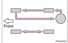
Do not fail to initialize the tire pressure warning system after tire rotation
