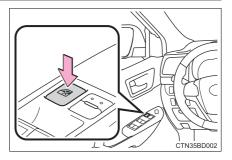
Models available with one touch opening/closing on all side windows: If the lock switch is on, the passenger windows can still be opened and closed using the power window switches on the driver's side.
