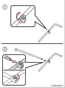
7 Connect the jack handle to the adapter socket. Turn the jack handle counterclockwise.
