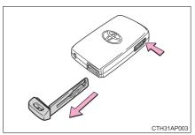
After using the mechanical key, store it in the electronic key. Carry the mechanical key together with the electronic key. If the electronic key battery is depleted or the entry function does not operate properly, you will need the mechanical key. ( $\rightarrow$ P. 517)
