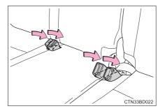
2 Pass the outer seat belts through the seat belt hangers and secure the seat belt plates.
