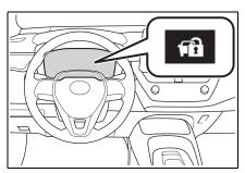
The indicator light flashes after the engine switch has been turned off to indicate that the system is operating.
