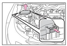
► Engine compartment: type B fuse box
