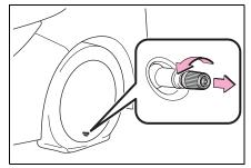
3 Extend the hose. Remove the air release cap from the hose.
