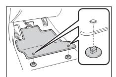
Turn the upper knob of each retaining hook (clip) to secure the floor mats in place.
