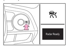
2 Accelerate or decelerate, with accelerator pedal operation, to the desired vehicle speed (at or above approximately 20 mph [30 km/h]) and press the "-SET" switch to set the speed. Cruise control "SET" indicator will come on.
