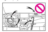
Do not attach anything to areas such as a door, windshield, side windows, front or rear pillar, roof side rail and assist grip. (Except for the speed limit label →P.468)
