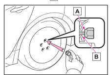
When replacing an aluminum wheel with a steel wheel, tighten the wheel nuts until the tapered portion A comes into loose contact with the disc wheel seat B
