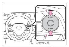
1 Increases the speed (Except when the vehicle has been stopped by system control in vehicle-to-vehicle distance control mode)
