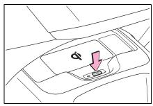
2 Place a portable device on the charging area with its charging surface facing down. While charging, the operation indicator light (orange) will be illuminated.
