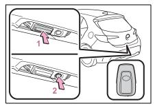
Press the button to unlock the back door.
