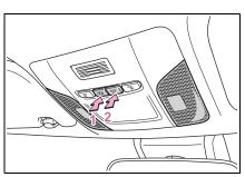
1 Turns the door position on/off When a door is opened while the door position is on, the lights turn on.
