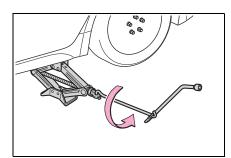
Firmly tighten each wheel nut two or three times in the order shown in the illustration.
