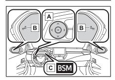
A Meter control switches Turning the Blind Spot Monitor
