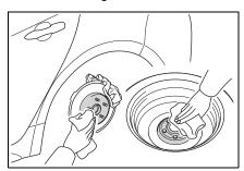
Install the tire and loosely tighten each wheel nut by hand by approximately the same amount.
