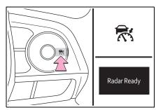
2 Accelerate or decelerate, with accelerator pedal operation, to the desired vehicle speed (at or above approximately 20 mph [30 km/h]) and press the "-SET" switch to set the speed.
