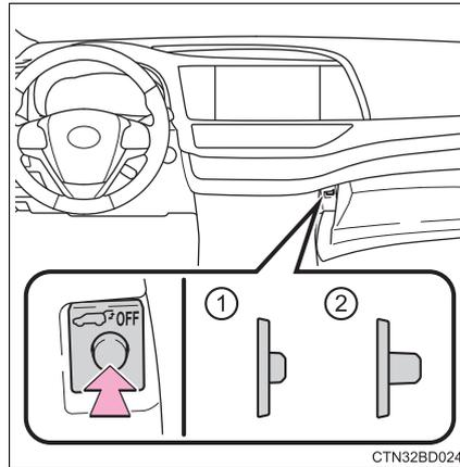
**Adjusting the open position of the back door (vehicles with a power back door)**
