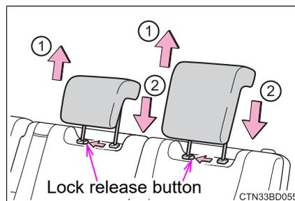
**■ Removing the head restraints****▶ Front seats and second seats (with a side table)**
