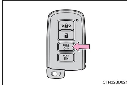
**Power back door switch (vehicles with a power back door)**
