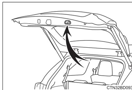
The back door closing assist will activate and the back door will fully close automatically.
