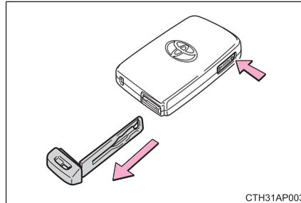
After using the mechanical key, store it in the electronic key. Carry the mechanical key together with the electronic key. If the electronic key battery is depleted or the entry function does not operate properly, you will need the mechanical key. (→P. 637)
