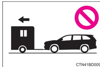
■ **To prevent causing serious damage to the transmission and the Dynamic Torque Control AWD system (AWD models)**
