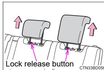
■ **Installing the head restraints**
