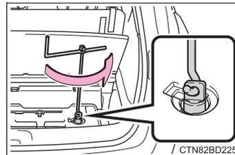
If the spare tire still cannot be lowered, the wire cable may be severed. Have the vehicle inspected by your Toyota dealer.
