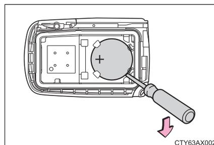
■ **Use a CR2016 (vehicles without a smart key system) or CR2032 (vehicles with a smart key system) lithium battery**
