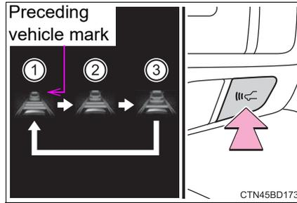
**Vehicle-to-vehicle distance settings (vehicle-to-vehicle distance control mode)**
