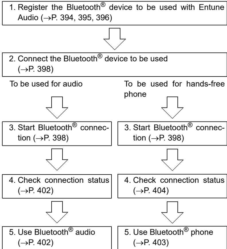
**Registering and connecting from the “Bluetooth\* Setup” screen**
