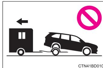
AWD models: Never tow this vehicle with any of the wheels on the ground. This may cause serious damage to the Dynamic Torque Control AWD system and transmission.
