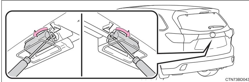
Insert a properly sized screwdriver into the hole of the lens on the inner side and disengage the claw and pry the lens toward the outer side as shown in the illustration.
