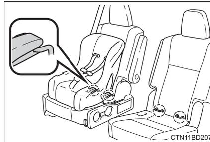
Seat belts equipped with a child restraint locking mechanism (ALR/ELR belts except driver's seat belt) (→P. 35)
