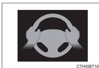
If the driver continues to keep their hands off of the steering wheel, a buzzer sounds and a warning message and the symbol shown in the illustration are displayed on the multi-information display. This warning also operates in the same way when the driver continuously operates the steering wheel only a small amount. Always keep your hands on the steering wheel when using this system, regardless of warnings.
