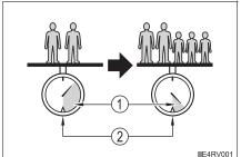
When 2 people with the combined weight of A lb. (kg) are riding in your vehicle, which has a total load capacity (vehicle capacity weight) of B lb. (kg), the available amount of cargo and luggage load capacity will be C lb. (kg) as follows:
