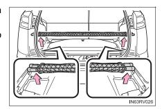
2 Push the right or left end of the pole into the slide rail.
