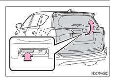
When the back door is locked (vehicles with smart key system): While carrying the electronic key on your person, press the back door opener switch.
