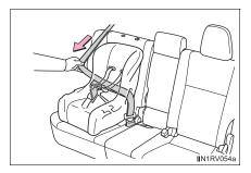
5 While pushing the child restraint system into the rear seat, allow the shoulder belt to retract until the child restraint system is securely in place.
