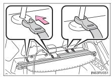
3 Pull out the luggage cover and hook it onto the anchors.
