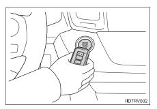
3 Firmly depress the brake pedal and check that on the multi-information display.
