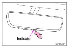
The function will set to ON mode each time the engine switch is turned to the "ON" position (vehicles without smart key system) or IGNITION ON mode (vehicles with smart key system).
