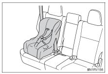
3 Latch the hook onto the anchor bracket and tighten the top tether strap.
