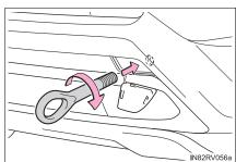
4 Tighten down the towing eyelet securely using a wheel nut wrench or hard metal bar.
