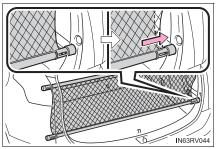
Align the other end of the pole with the corresponding fixed position on the other side and release the pole.
