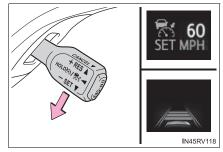
The vehicle speed at the moment the lever is released becomes the set speed.
