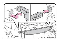
2 For vehicles with hooks: Attach the hooks to the rear seat head restraints.
