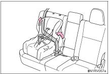
6 If the child restraint has a top tether strap, the top tether strap should be latched onto the top tether strap anchor.  $(\rightarrow P. 69)$
