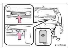
② Press the button to lock all the doors. Check that the door is securely locked.
