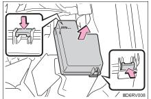
Push the tabs in and lift the cover off.
