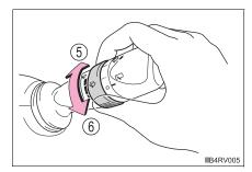
Washer/wiper dual operation The wipers will automatically operate a couple of times after the washer squirts.
