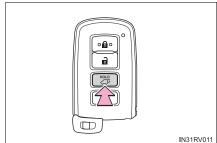
Pressing the button while the back door is opening/closing stops the operation.
