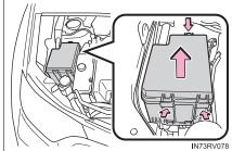
Push the tabs in and lift the cover off.
