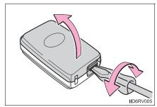
3 Remove the depleted battery.
