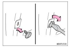
9 Reinstall the fender liner and install the screws.
