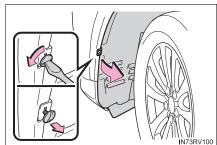
4 Unplug the connector while pressing the lock release.
