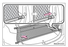
2 Perform the steps 2 and 3 in "Installing the rear cargo net". (→P. 520)
