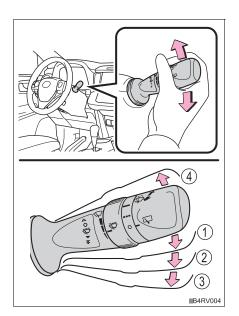
If equipped, wiper intervals can be adjusted when intermittent operation is selected.
