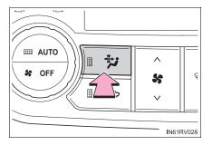
Defoggers are used to defog the windshield and front side windows.
