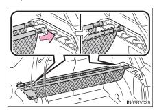
2 Slide the pole to the desired fixed position, and push down.
