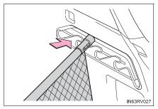
Push the other end of the pole into the slide rail, and then install both ends into fixed positions.
