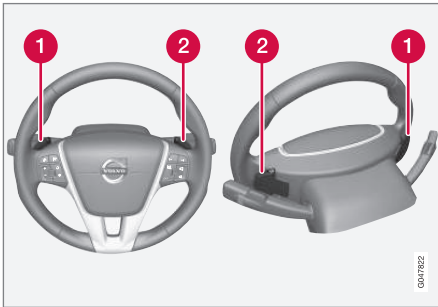
Steering-wheel mounted gear shift paddles
