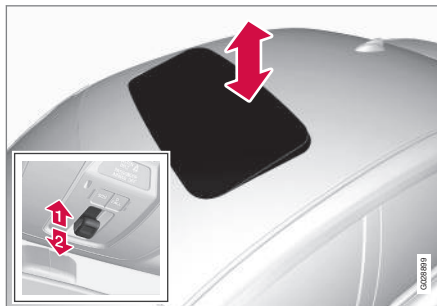
Tilt position, raised at the rear edge
