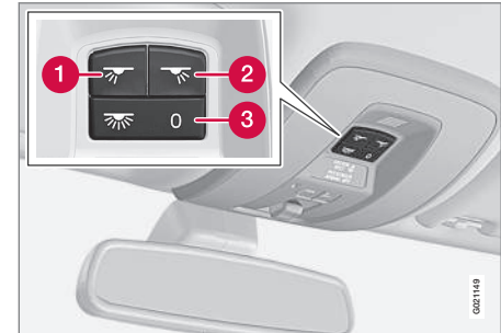
Light switches, front roof lighting
