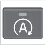
Start/Stop button on the center console
