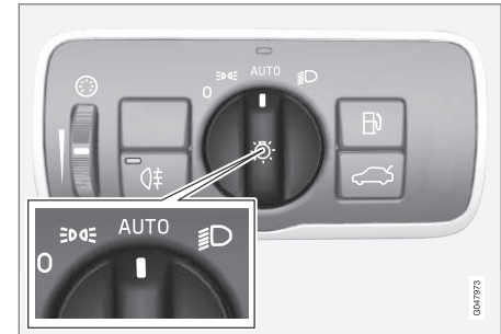
Headlight switch in the AUTO position
