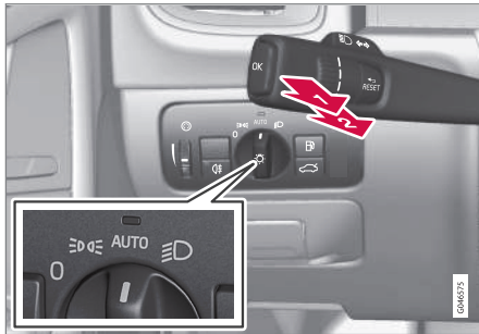
Headlight switch and steering wheel lever
