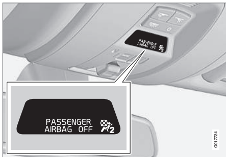
Occupant Weight Sensor (OWS) indicator light
