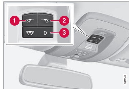
Light switches, front roof lighting
