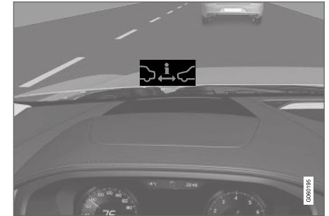
Distance Alert warning symbol on the windshield 32 .
