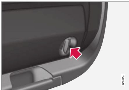
Left-side bulb housing.
