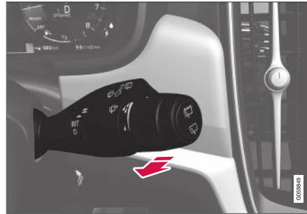
Washing function, right-hand steering wheel lever.
