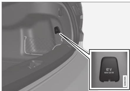
12 V outlet in trunk/cargo compartment*.
