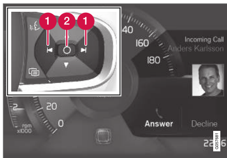
Messages in the instrument panel 6 and the right-side steering wheel keypad.
