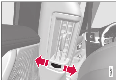
Air vent thumb wheel 2 .
