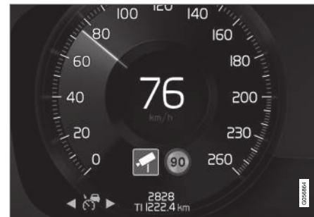
Speed camera information in the instrument panel 98 .
