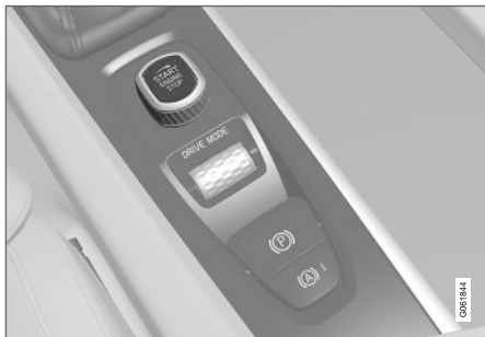
Start knob in the tunnel console.
