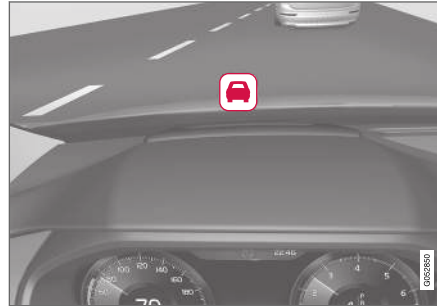
Collision warning symbol on the windshield 57 .
