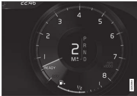
Manual shifting mode in the instrument panel 2 .
