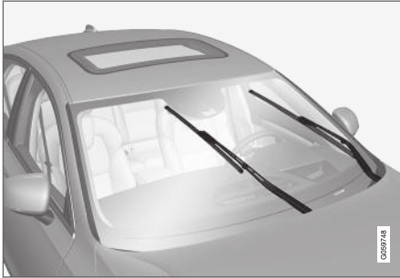
Windshield wipers in the service position.
