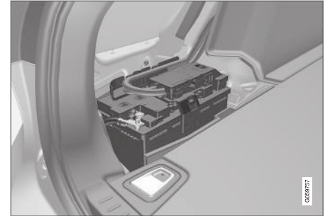
The start battery is located in the cargo compartment.
