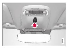
The panoramic roof and sun curtain are operated using the controls in the ceiling.
