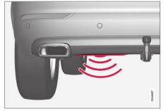
The sensor is located to the left of center under the rear bumper.
