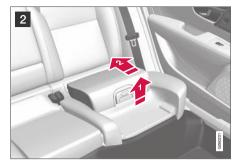
Lift the front edge of the booster cushion and press it rearward toward the backrest to lock it into position.
