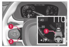
Controls for setting a time interval<sup>58</sup>.
