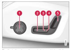
The illustration shows the controls in a vehicle with fourway lumbar support\*. Vehicles with two-way lumbar support\* do not have the rotary multifunction control.
