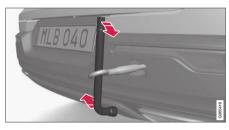
Fasten the eyelet securing by, for example, inserting a lug wrench\* through it and using this as a lever.
