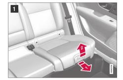
Pull the handle forward and upward to release the booster cushion.
