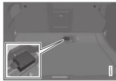
Insert a personal SIM card in the holder under the floor of the cargo compartment.
