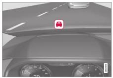
Collision warning symbol on the windshield<sup>70</sup>.
