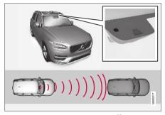
Location of the camera and radar sensor<sup>68</sup>.
