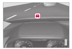
Collision warning symbol on the windshield<sup>39</sup>.
