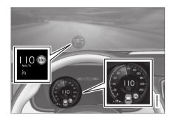
The previous illustration<sup>54</sup> shows that Adaptive Cruise Control is set to maintain a speed of 110 km/h (68 mph) and that there is no target vehicle ahead to follow.
