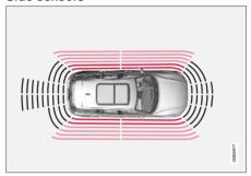
Rapid pulsing warning signal when the obstacle is less than approx. 25 cm (0.8 ft) from the vehicle <sup>110</sup>.
