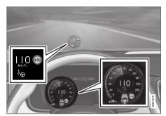
The previous illustration<sup>62</sup> shows that Pilot Assist is set to maintain a speed of 110 km/h (68 mph) and that there is no target vehicle ahead to follow.
