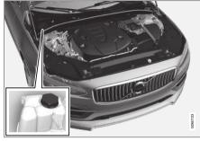
Coolant expansion tank, left-hand drive vehicle.
