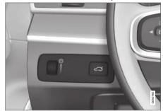
Thumb wheel (to the left) for adjusting interior brightness.
