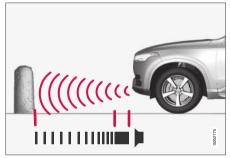
Continuous tone warning signal when the obstacle is less than approx. 30 cm (1 ft) from the vehicle <sup>110</sup>.
