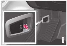
Pull the lever near the pedals to release the hood from its fully closed position.
