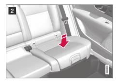
Press down on the center of the booster cushion to lock it into position.
