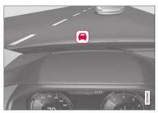
Collision warning symbol on the windshield<sup>57</sup>.
