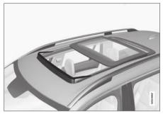
The panoramic roof is equipped with a wind blocker that folds up when the roof is open.
