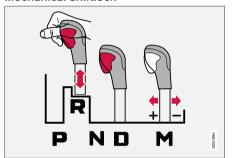
The gear selector can be moved back and forth between  ${\bf N}$  and  ${\bf D}$ . The other positions have a shiftlock that is operated using the lock button on the gear selector.
