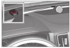
A red LED light on the dashboard will flash every other second when the vehicle is locked and the alarm is armed.
