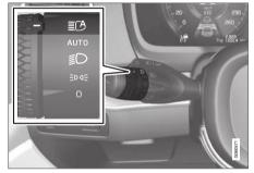
Active high beam is enabled by moving the lighting ring on the steering wheel lever to AUTO.
