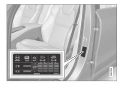
The decal specifies the designation for the factory-mounted tires on the vehicle, as well as load limits and inflation pressures.
