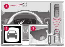
Collision warning audible signal and symbol<sup>56</sup>.
