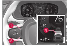
Controls for setting a time interval<sup>43</sup>.
