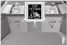
Top tether anchors and symbols on the rear side of the rear seat backrests. There is no symbol for the center anchor position.
