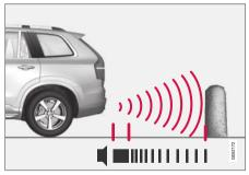
Continuous tone warning signal when the obstacle is less than approx. 30 cm (1 ft) from the vehicle <sup>110</sup>
