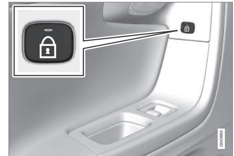
The indicator light in the button is on when the door is locked
