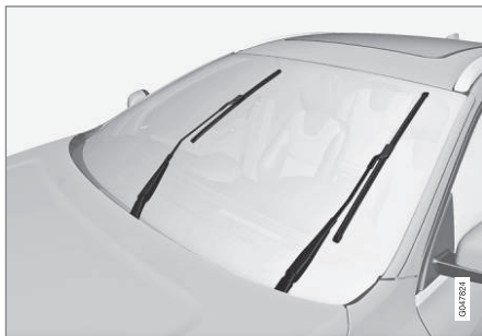
Wiper blades in service position
