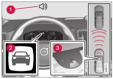
Collision warning audible signal and symbol<sup>62</sup>.
