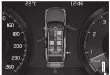
Graphics in the instrument panel with various types of warnings. The warning colors for the doors/tailgate vary depending on the vehicle's speed.
