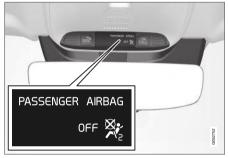
Occupant Weight Sensor (OWS) indicator light
