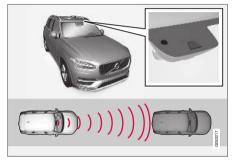
The camera/radar sensor measures the distance to the vehicle ahead<sup>41</sup>.
