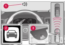
Collision warning audible signal and symbol<sup>42</sup>.
