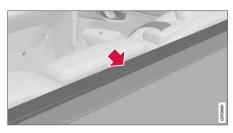
Fold out the cover's front flap to eliminate the gap between the cover and the rear seat backrest.
