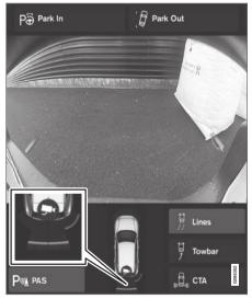
The screen can display colored sensor fields on the vehicle symbol <sup>121</sup>.
