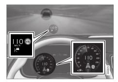
The previous illustration <sup>68</sup> shows that Pilot Assist is set to maintain a speed of 110 km/h (68 mph) and is following a target vehicle ahead that is traveling at the same speed.
