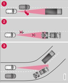
The radar sensor's field of vision.
