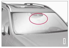
The area marked in the illustration must be kept free of decals, objects, solar film, etc.  $^{73}$
