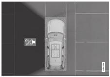
The vehicle's left-side camera is malfunctioning.
