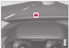
Collision warning symbol on the windshield<sup>63</sup>
