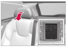
The outer head restraints can be folded via the center display's function view. The head restraint can be folded down when the vehicle is in ignition mode  $\bf 0$ .
