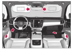
Storage compartment in the door panel and near the steering wheel, glove compartment and sun visors.
