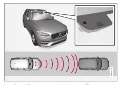
Location of the camera and radar sensor<sup>74</sup>.
