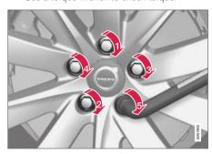
5. Press the plastic covers onto the wheel bolts.
