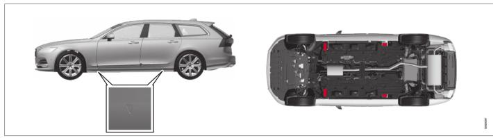
The triangles in the plastic covering indicate where the jack attachment points/lifting points (red areas) are located.
