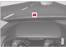
Collision warning symbol on the windshield<sup>43</sup>.
