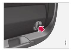
Remove the panel on the inside of the tailgate by turning both clips counterclockwise a quarter-turn. Remove the panel. Place the panel in a safe location out of the way.
