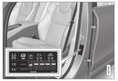
The placard specifies the designation for the factory-mounted tires on the vehicle, as well as load limits and inflation pressures.
