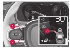
Controls for setting a time interval.
