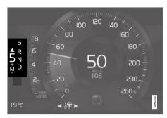
Gear indicator in 8" instrument panel.
