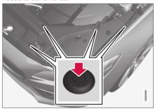
Release the pins in the plastic cover's four clips by pressing them down with a screwdriver or similar object and remove the covering.
