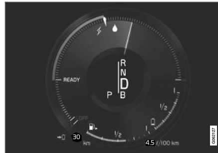
The instrument panel gauge when both the electric motor and the combustion engine are being used.
