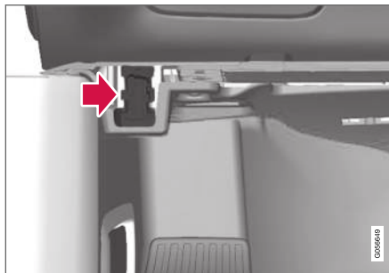
On-board Diagnostic (OBDII) socket under the dashboard on the driver's side.
