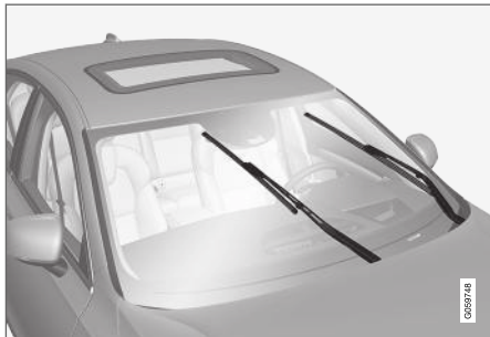
Windshield wipers in the service position.
