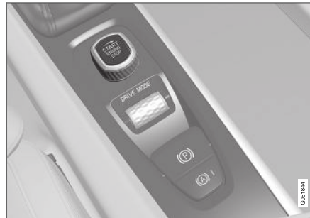
Start knob in the tunnel console.
