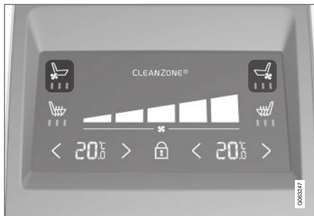
Seat ventilation controls and indicator lights on the rear side of the tunnel console.
