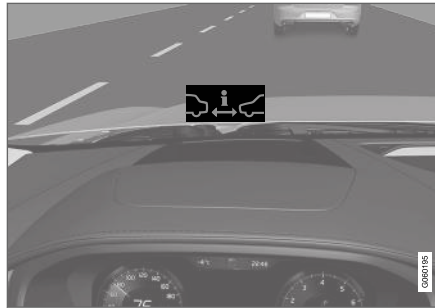
Distance Alert warning symbol on the windshield 33 .
