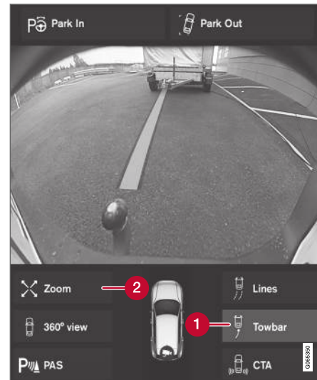
Towbar with trajectory line 117 .
