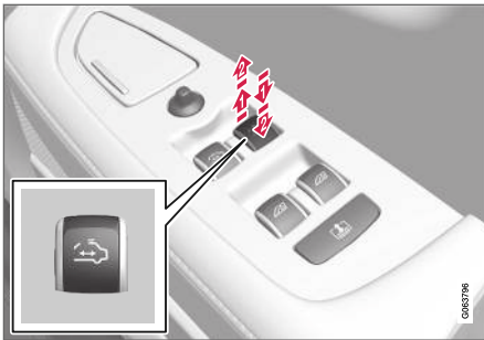
Panoramic roof control.
