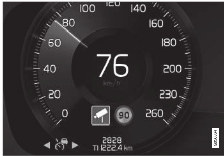
Speed camera information in the instrument panel 99 .
