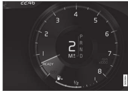
Manual shifting mode in the instrument panel 2 .
