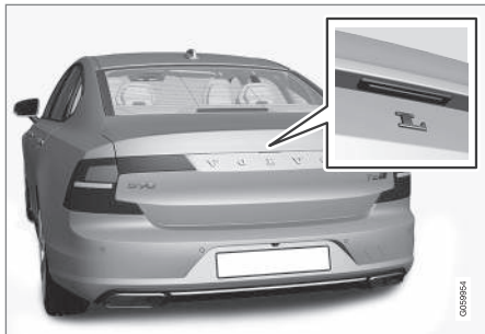
Rubberized button on the trunk used only for unlocking
