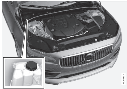
Coolant expansion tank
