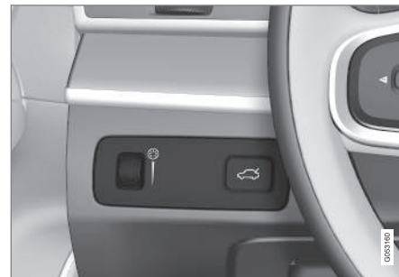
Thumb wheel (to the left) for adjusting display brightness
