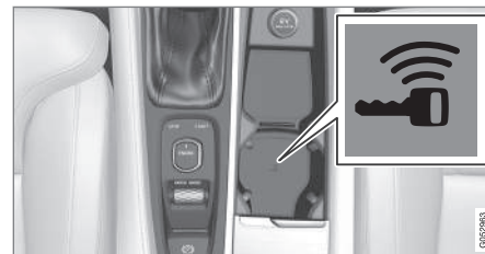
Back-up reader in the tunnel console
