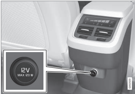
12-volt socket in the tunnel console for the rear seats
