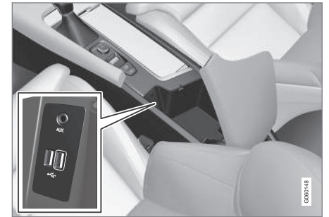
AUX/USB sockets in the tunnel console
