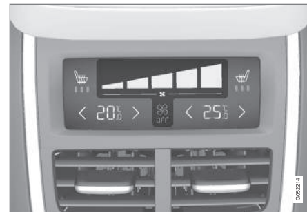
Blower controls on the climate panel on the rear side of the tunnel console
