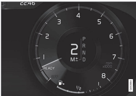
Manual shift indicator in the instrument panel 8 .
