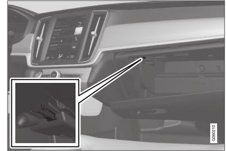
Storage compartment for the key. The illustration is generic – the design may vary.
