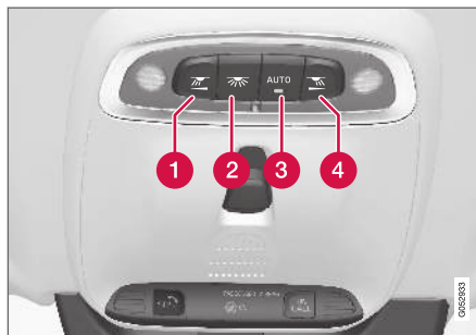
The controls in the ceiling console for the front reading lights and courtesy lighting.
