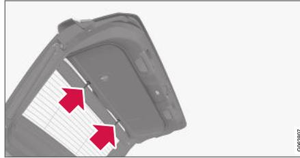
**Removing the cargo compartment cover**
