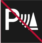
Be extra cautious when reversing if this symbol is shown when a trailer, bike carrier or similar is attached and electrically connected to the vehicle.
