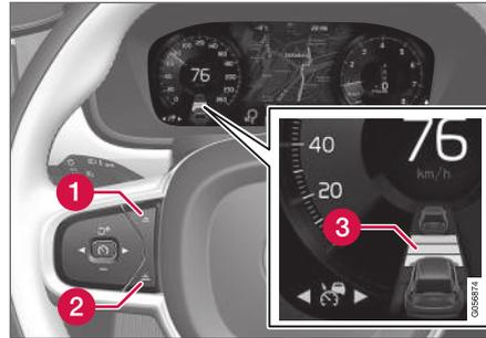
Controls for setting a time interval<sup>47</sup>.
