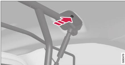
4. Screw the provided screw into place using the provided 6 mm Allen wrench. Repeat on the other side. Recommended torque: 20 Nm (15 ft-lb).
