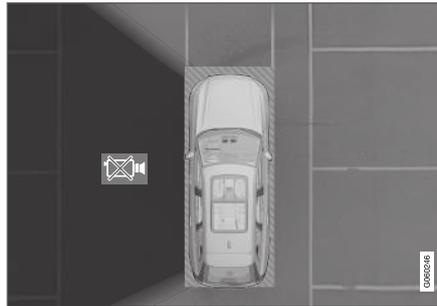
The vehicle's left-side camera is malfunctioning.
