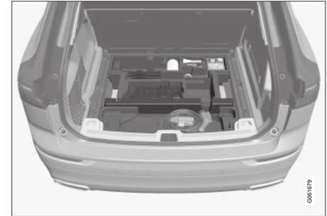
The foam block under the cargo compartment floor contains the towing eyelet, the tire sealing system, the tool for removing plastic wheel bolt covers and the tool for removing the locking wheel bolts.
