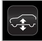
The instrument panel indicates when the suspension level is being adjusted.
