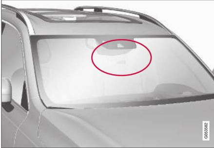
The area marked in the illustration must be kept free of decals, objects, solar film, etc.<sup>69</sup>
