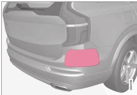
Keep this area clean (on both the left and right sides of the vehicle)<sup>83</sup>.
