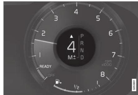
Gear indicator in 12" instrument panel\*.
