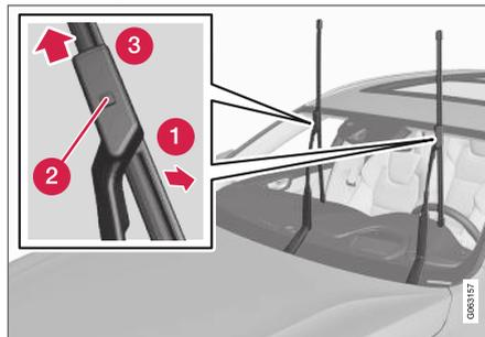
1. Raise the wiper arms to the service position. Service position is activated/deactivated via the function view in the center display when the car is stationary and the windshield wipers are not on.
