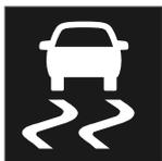
When Trailer Stability Assist is activated, the **ESC** symbol is displayed in the instrument panel.
