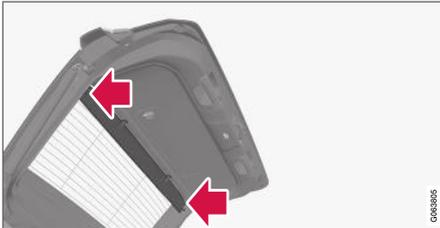
2. Squeeze together the flap slightly to make it easier to guide the pin into place in the bracket on the other side.
