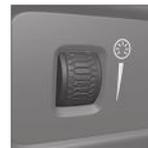
The thumb wheel on the dashboard at the steering wheel can be used to adjust the brightness of the display lighting, instrument lights, ambient lighting and mood lighting\*
