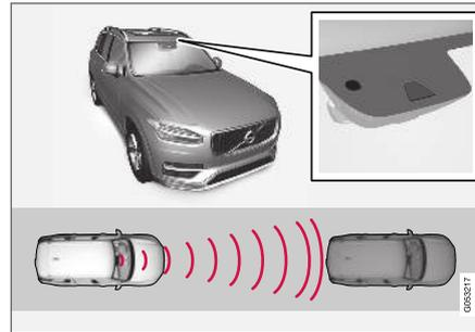
Location of the camera and radar sensor<sup>74</sup>.
