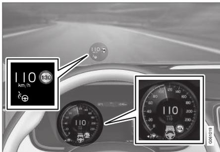
The previous illustration<sup>68</sup> shows that Pilot Assist is set to maintain a speed of 110 km/h (68 mph) and that there is no target vehicle ahead to follow.
