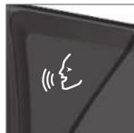
Press the button for voice control
