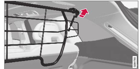
3. Position the grid's attachment points in the ceiling consoles.
