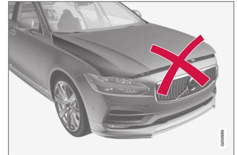
Hood not completely closed. The illustration is generic - details may vary according to vehicle model.
