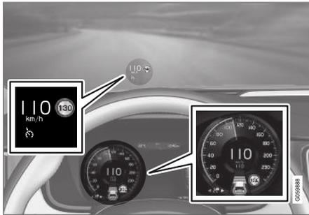
The previous illustration<sup>60</sup> shows that Adaptive Cruise Control is set to maintain a speed of 110 km/h (68 mph) and that there is no target vehicle ahead to follow.
