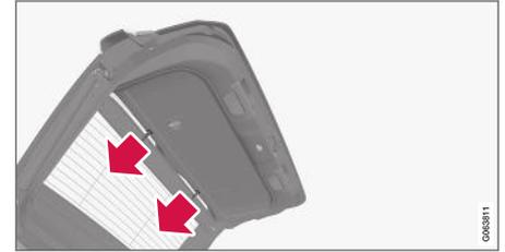
2. Carefully pull the flap out of the bracket on one side of the tailgate and then the other. If necessary, press the flap together slightly to make it more flexible and facilitate removal.
