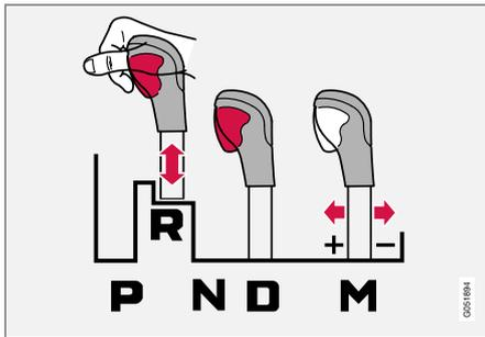
The gear selector can be moved back and forth between **N** and **D**. The other positions have a shiftlock that is operated using the lock button on the gear selector.
