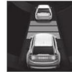
ACC will only regulate the time interval to the vehicle ahead when the distance symbol shows two vehicles.
