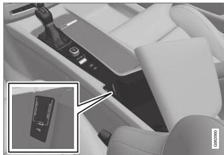
USB ports (type A) in the tunnel console. Route the cable forward to help avoid pinching when the cover is closed.
