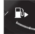
An arrow next to the fuel pump symbol in the instrument panel indicates the side of the vehicle on which the fuel filler door is located.
