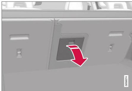
1. In the cargo compartment, grasp the ski hatch handle and pull it down.
