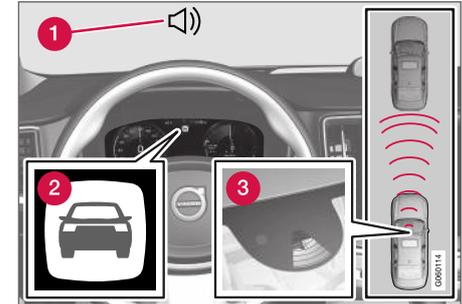
Collision warning audible signal and symbol<sup>62</sup>.
