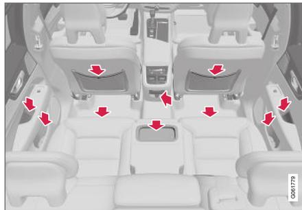
Storage compartment in the door panel, cup holders\* in the center seat's backrest, storage pocket\* in the front seat's backrest, electrical outlets in the tunnel console and storage compartment under the seat.
