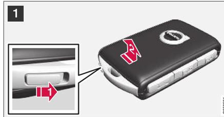
**1** ➔ Hold the remote key with the front side (with the Volvo logo) facing up and move the button on the key ring section to the right. Slide the front cover slightly upward.
