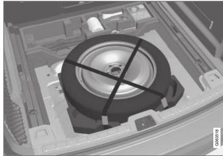
The spare wheel is located under the floor of the cargo compartment and is held in place by two straps. The foam block contains all tools needed to change a wheel.
