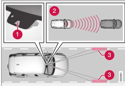
The camera/radar sensor monitors the distance to the vehicle ahead and detects lane markings<sup>61</sup>.
