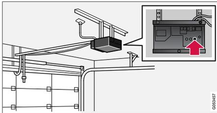
4. Locate the "training" button<sup>14</sup> on the receiver for the e.g. garage door opener. It is usually located near the antenna bracket on the receiver.
