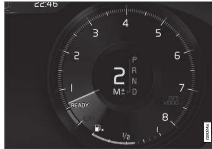
Manual shifting mode in the instrument panel<sup>2</sup>.
