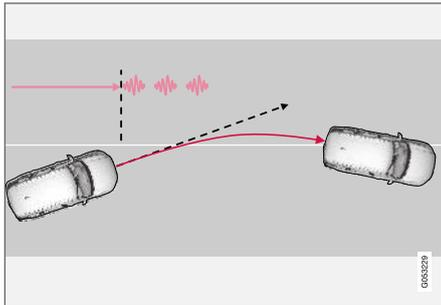
Lane Keeping Aid alerts the driver using vibrations in the steering wheel<sup>107</sup>.
