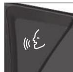
The voice control system enables the driver to control certain vehicle functions without taking their hands off the wheel. The system can understand natural speech. Use voice commands to e.g. play a song, make a phone call, increase the temperature in the passenger compartment or have a text message read aloud.
