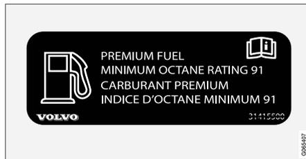
Decal on the inside of the fuel filler flap on cars that require premium fuel<sup>8</sup>.
