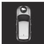
The active cameras will be indicated by a camera symbol on the vehicle symbol in the center display.
