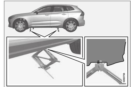
9. Position the jack under the attachment point being used, ensuring that the surface is firm, flat and not slippery.
