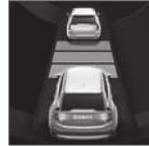
Different time intervals to the vehicle ahead can be selected and are shown in the instrument panel as 1–5 horizontal bars. The more bars, the longer the time interval. One bar represents an interval of
