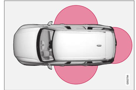
The shaded areas around the vehicle illustrate the range of the system's antennas.
