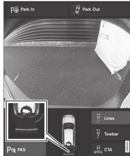
The screen can display colored sensor fields on the vehicle symbol<sup>121</sup>.
