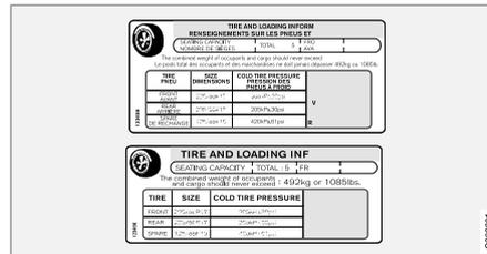
**3 Tire inflation pressures.** This label indicates the correct inflation pressures for the tires that were on the vehicle when it left the factory.
