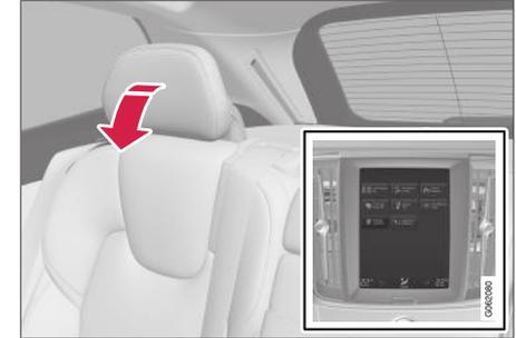
The outer head restraints can be folded via the center display's function view. The head restraint can be folded down when the vehicle is in ignition mode **O**.
