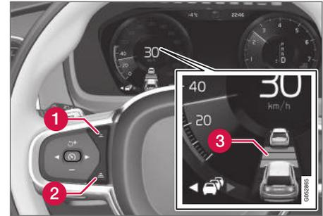
Controls for setting a time interval.
