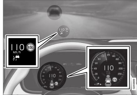
The previous illustration<sup>60</sup> shows that Adaptive Cruise Control is set to maintain a speed of 110 km/h (68 mph) and is following a target
