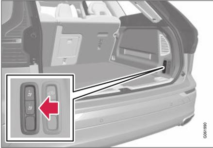
On models equipped with the electric fold-down function\*, the buttons for folding down the rear seat backrests are located in the cargo compartment. The backrests can also be folded down manually.
