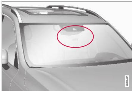
The area marked in the illustration must be kept free of decals, objects, solar film, etc.<sup>73</sup>
