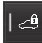
The function button for private locking is located in the center display's Function view. Depending on the current status of the lock, **Private Locking Unlocked** or **Private Locking Locked** will be displayed.
