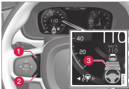
Controls for setting a time interval<sup>64</sup>.
