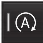
To turn off Start/Stop, tap the **Start/Stop** function button in the center display's Function view. The indicator light in the button will go out when the function has been turned off.
