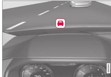
Collision warning symbol on the windshield<sup>63</sup>.
