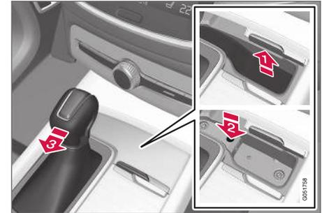
If the vehicle cannot be driven (e.g. due to a discharged battery), the gear selector must be moved to the **N** position so that the vehicle can be moved.
