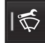
Tap the **Wiper Service Position** button. The indicator light in the button will illuminate when service position is activated. The windshield wipers will move to the vertical position when service position is activated. To deactivate the service position, tap **Wiper Service Position** once. The indicator light in the button will go out when service position is deactivated.
