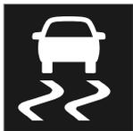
This symbol will be displayed in the instrument panel when the ESC system is intervening.
