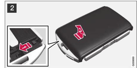
**2** ➔ Turn the key over, move the button to the side and slide the rear cover slightly upward.
