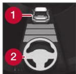
Pilot Assist's steering assistance is only active when the steering wheel symbol (2) changes from GRAY to GREEN.
