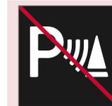
Be extra cautious when reversing if this symbol is shown when a trailer, bike carrier or similar is attached and electrically connected to the vehicle.
