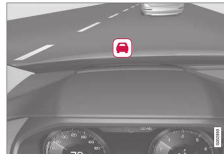
Collision warning symbol on the windshield<sup>43</sup>.
