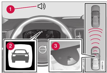
Collision warning audible signal and symbol<sup>42</sup>.
