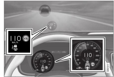
The previous illustration<sup>68</sup> shows that Pilot Assist is set to maintain a speed of 110 km/h (68 mph) and is following a target vehicle ahead that is traveling at the same speed.
