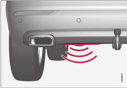
The sensor is located to the left of center under the rear bumper<sup>18</sup>.
