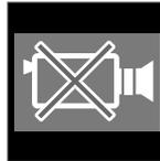
If a camera sector is dark and contains this symbol, this indicates that the camera is not functioning properly.
