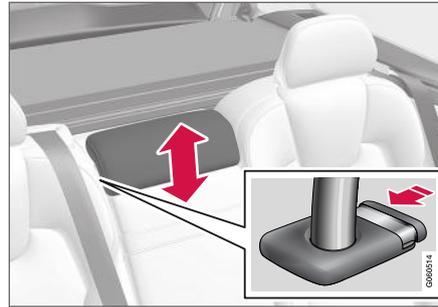
To lower the restraint, push and hold the button (see illustration) while carefully lowering the head restraint.
