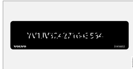
**2 Vehicle Identification Number (VIN).** The VIN plate is located on the top left surface of the dashboard. The Vehicle Identification Number (VIN) should always be quoted in all correspondence concerning your vehicle with the retailer and when ordering parts.
