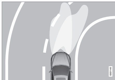
Headlight pattern with the Active Bending Light function deactivated (left) and activated (right)
