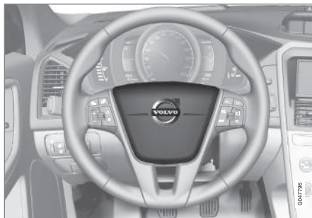
Button for steering wheel heating
