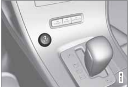
12-volt socket in the front tunnel console
