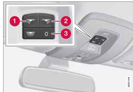
Light switches, front roof lighting
