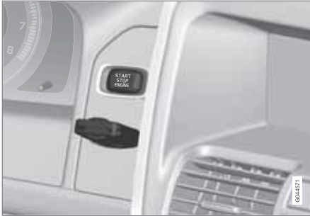
Ignition switch with remote key inserted ( see page 81 for more information on ignition modes)
