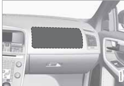
Location of the passenger's side front airbag
