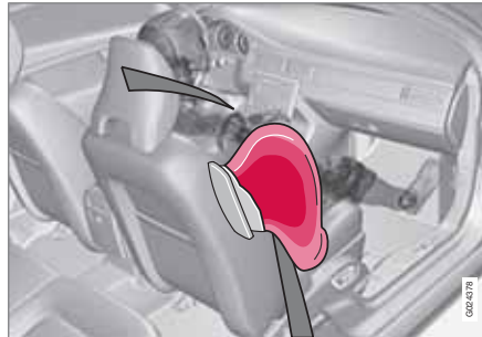
Passenger's side SIPS airbag
