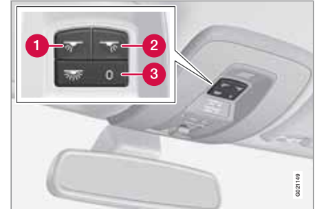
Light switches, front roof lighting
