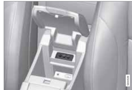
The A/V-AUX socket is located under the center armrest in the tunnel console
