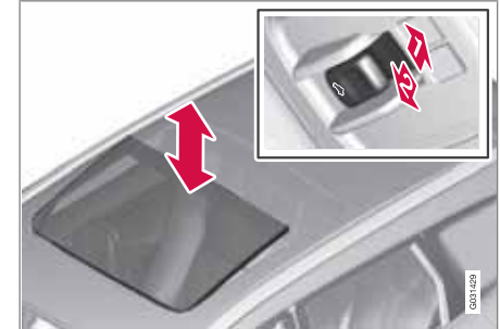
Tilt position, raised at the rear edge
