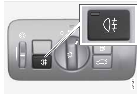
Headlight control in position for parking lights
