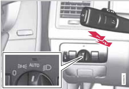
Headlight switch with AUTO and lever
