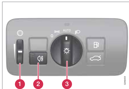
Overview, light switches with AUTO function
