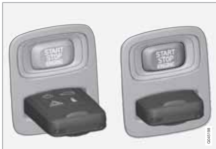
Ignition slot with remote key inserted ( see page 84 for more information on ignition modes)
