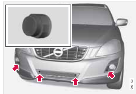
Location of the front sensors
