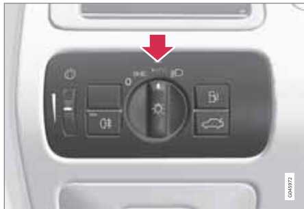
Light switch in the AUTO position
