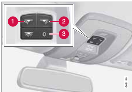
Light switches, front roof lighting
