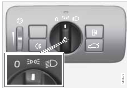
Headlight control in position for parking lights
