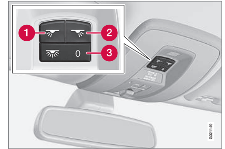
Light switches, front roof lighting
