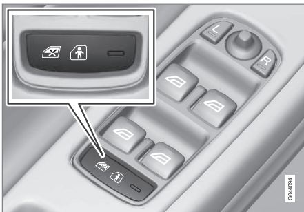
Driver's door control panel
