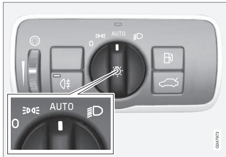
Headlight switch in the AUTO position
