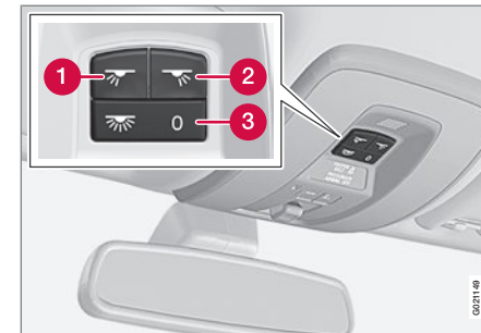
Light switches, front roof lighting
