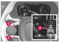
Controls for setting a time interval<sup>60</sup>.
