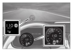
The previous illustration  $^{64}$  shows that Pilot Assist is set to maintain a speed of 110 km/h (68 mph) and that there is no target vehicle ahead to follow.
