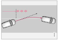
Lane Keeping Aid alerts the driver using vibrations in the steering wheel  $^{\rm 105}\!$
