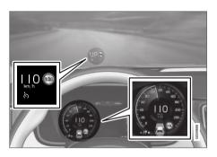
The previous illustration<sup>56</sup> shows that Adaptive Cruise Control is set to maintain a speed of 110 km/h (68 mph) and that there is no target vehicle ahead to follow.
