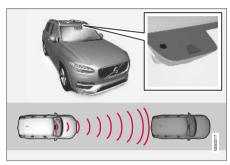
Location of the camera and radar sensor<sup>70</sup>.
