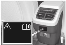
Electrical outlet in the tunnel console, second row of seats.
