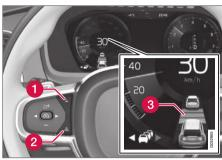
Controls for setting a time interval.
