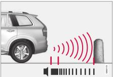
Continuous tone warning signal when the obstacle is less than approx. 30 cm (1 ft) from the vehicle  $^{112}\,$
