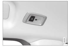
In vehicles with panoramic roofs\*, there are two lamp units, one on each side of the ceiling.<sup>7</sup>
