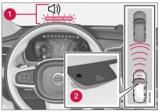
Collision warning light on the windshield<sup>58</sup>.
