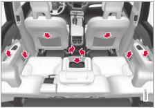
Storage compartment in the door panel, cup holders\* in the center seat's backrest, storage pocket\* in the front seat's backrest and electrical outlets in the tunnel console.
