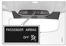
Occupant Weight Sensor (OWS) indicator light
