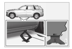
Position the jack under the attachment point being used, ensuring that the surface is firm, flat and not slippery.
