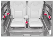
Storage compartment and cup holders in the side panel and storage compartment between the seats.
