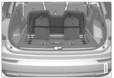
There are two grocery bag holders and an elastic band<sup>4</sup> in the hatch in the cargo compartment floor. The strap can be attached in four different positions.
