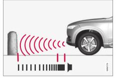
Continuous tone warning signal when the obstacle is less than approx. 30 cm (1 ft) from the vehicle  $^{112}\!\!$
