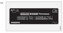
**6** Engine oil. This label contains the recommended engine oil specifications.
