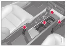
Storage compartments with cup holders, net pocket\*, electrical outlets and USB ports in the tunnel console.
