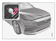
Yurn the handle under the front edge of the hood counterclockwise to release the catch and lift the hood.
