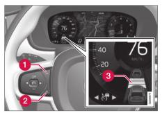
Controls for setting a time interval<sup>45</sup>.
