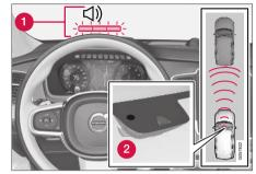
Collision warning light on the windshield<sup>40</sup>.
