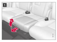
Pull the handle forward and upward to release the booster cushion.
