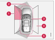
Parking sensor sectors where obstacles can be detected<sup>120</sup>.
