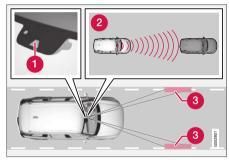
The camera/radar sensor monitors the distance to the vehicle ahead and detects lane markings<sup>57</sup>.
