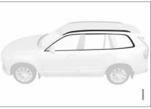
Components that should be washed with a cleaning product with a pH value between 3.5 and 11.5.
