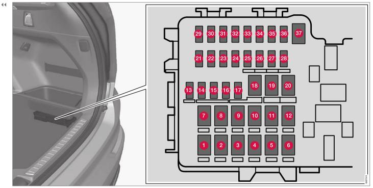
The fuse box is located under the storage compartment on the right-hand side.
