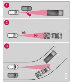
The radar sensor's field of vision.
