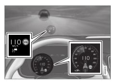
The previous illustration<sup>64</sup> shows that Pilot Assist is set to maintain a speed of 110 km/h (68 mph) and is following a target vehicle ahead that is traveling at the same speed.
