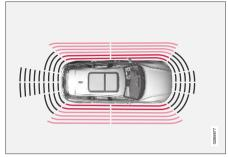
Rapid pulsing warning signal when the obstacle is less than approx. 25 cm (0.8 ft) from the vehicle  $^{112}$ .
