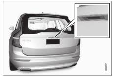
Rubberized pressure plate on the tailgate used only for unlocking.
