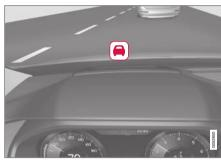
Collision warning symbol on the windshield<sup>59</sup>.
