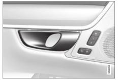
Alternative unlocking method using side door opening handle  $^{15}\!\!\!\!$
