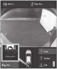
The front and rear fields change colors (from YELLOW to ORANGE to RED) as the vehicle moves closer to an obstacle.
