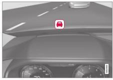
Collision warning symbol on the windshield<sup>72</sup>.
