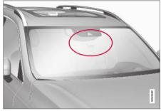
The area marked in the illustration must be kept free of decals, objects, solar film, etc.  $^{65}$
