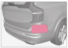
Keep the marked area clean (on both the left and right sides of the vehicle)  $^{88}$ .
