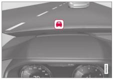
Collision warning symbol on the windshield<sup>41</sup>.
