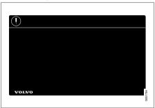
White ISO symbols and white text/image on a black or blue warning field and message field. Used to indicate potential danger. Ignoring a warning of this type could result in damage.
