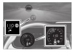
The previous illustration<sup>56</sup> shows that Adaptive Cruise Control is set to maintain a speed of 110 km/h (68 mph) and is following a target vehicle ahead, which is traveling at the same speed.
