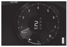
Manual shifting mode in the instrument panel<sup>2</sup>.
