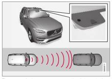
The camera/radar sensor measures the distance to the vehicle ahead  $^{\rm 39}\!.$
