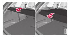
Grasp the handle and pull the cover out and above the side panels in the cargo compartment. Pull the cover to its end position.
