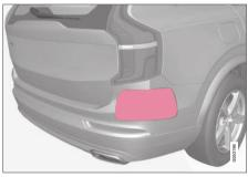
Keep the marked area clean (on both the left and right sides of the vehicle)  $^{80}\!\!.$
